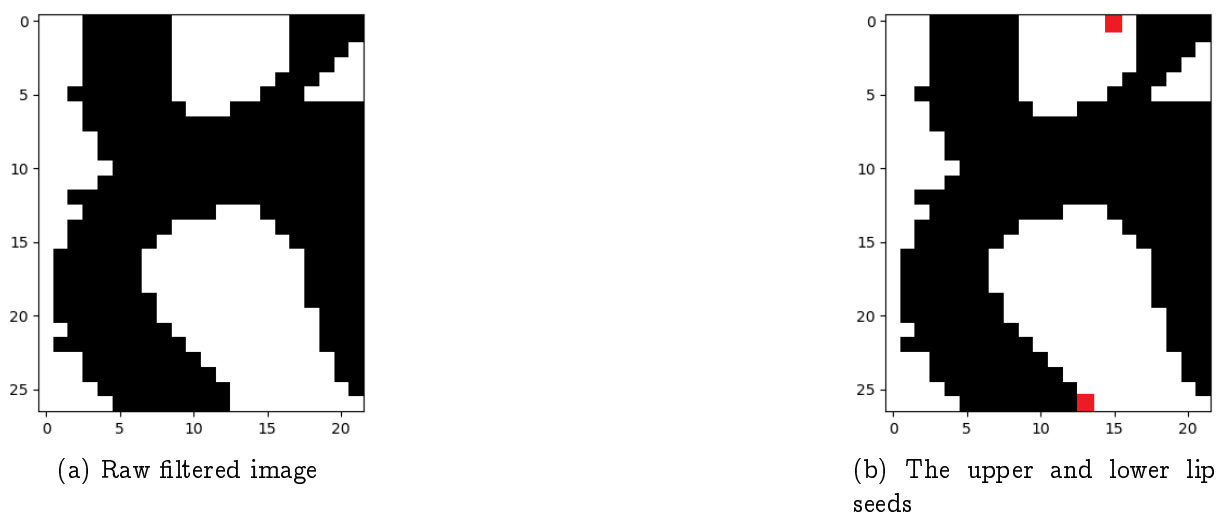
Figure 4.8: A sample image to extract articulatorily relevant information from the lips. The leftmost white area corresponds to the end of the vocal-tract-related part of the image and is thus irrelevant. The two elongated shapes in the center are the lips. There is the tongue tip approaching the upper lip at the right. The seed points are indicated in red.
