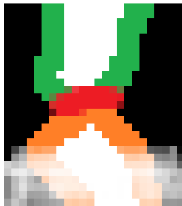
(e) ls\_cont is the distance between the outer and the inner contour, disregarding the lower 20% of the image (whitened out) that could produce a smaller distance.
