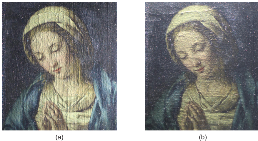
Figure 5.22: White-light raking images of Vièrge en priere with the light source (a) placed on the left side and (b) the top side of the painting.
