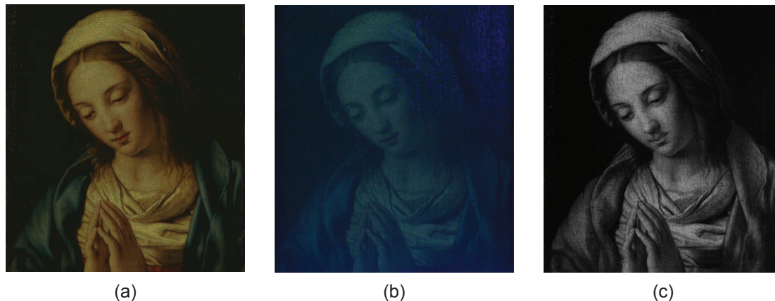
Figure 5.13: Images of Vierge en priere . (a) Visible photograph of the Viège en priere ; Image of Viège en priere obtained by UV Fluorescence; (c) Image of Viège en priere obtained by IR Reflectography.
