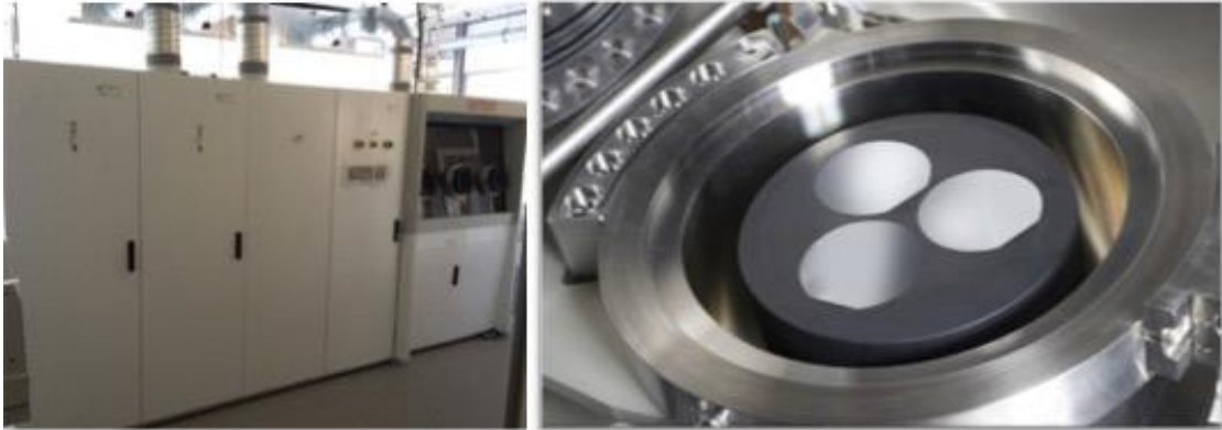
Figure 2-4 Aixtron 3x2 inch, close coupled showerhead (CCS) MOVPE system.
