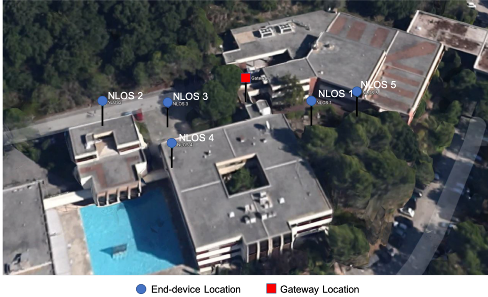
FIGURE 3.14: Outdoor Experiment testbed deployed on Inria campus showing the end-device locations (blue circles) and the gateway locations (red squares). The testbed is designed to evaluate Snipe in an outdoor environment rich with multipath and in NLoS propagation conditions.
