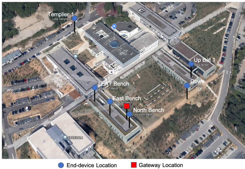
FIGURE 3.13: Experiment testbed showing the end-device locations (blue circles) and the gateway locations (red squares). The testbed is designed to evaluate Snipe in outdoor LoS condition with large building, cars and vegetation.
