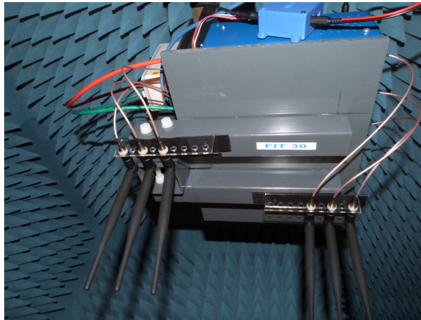
FIGURE 5.3: Wi-Fi dual-band antennas for a node
