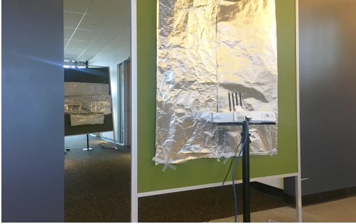
FIGURE 4.6: NLoS setup between a Tx and a subject.
