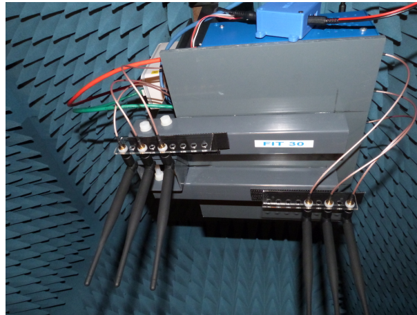
FIGURE 5.3: Wi-Fi dual-band antennas for a node
