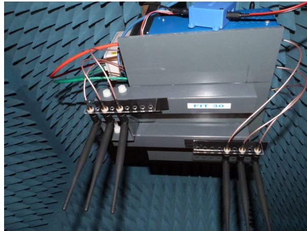
FIGURE 5.3: Wi-Fi dual-band antennas for a node
