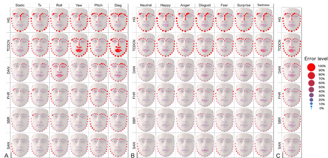
Figure 3.11: Heatmaps of landmark detection error (A: per head pose, B: per facial expression, C: in all). Eyebrows, facial edges, and the mouth are among the regions that are the most affected by head pose and facial expression.
