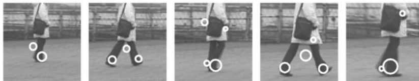
Figure 4.1: Space-time interest points detection [117]. The detected points are characterized by large variation of the image values in all three directions altogether, i.e., spatio-temporal corners.
