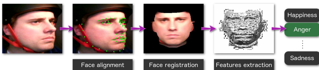
Figure 3.1: Typical facial expression recognition process. It relies on landmarks to normalize the face and extract appearance, geometry or motion features.
