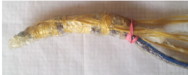
(a) Finger with tendons wrapped in film of SEBS-paraffin gel forming the subcutis.
