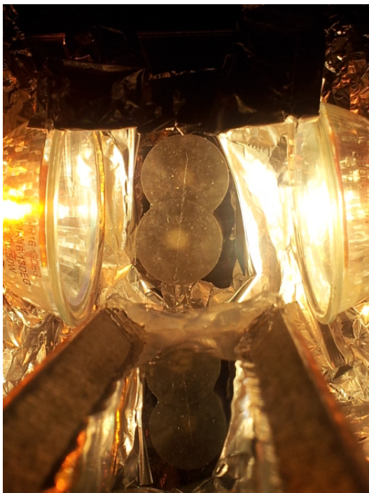
(c) Horizontal drawing over water - an experiment to draw SEBS fibres with GaIn filled channels
