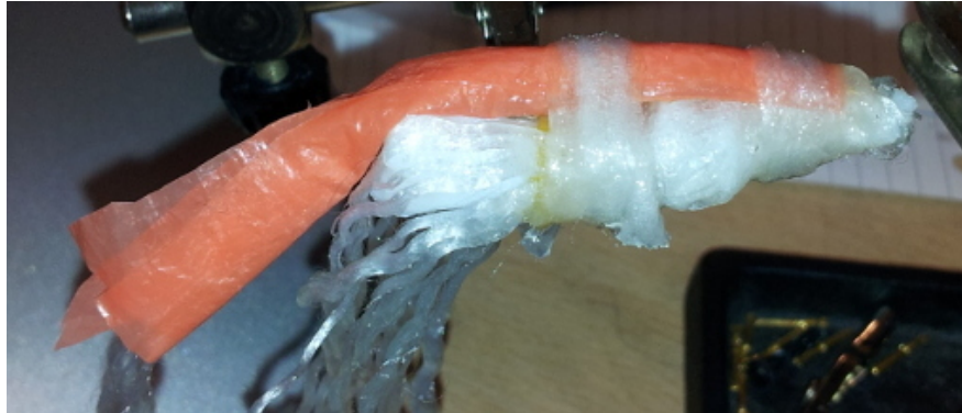
Figure 9-1: First test flexor tendon sheath - polyamide tendon with silicone gel matrix and silicone oil tendon fluid, high density polyethylene sheath, polyamide annular ligaments with silicone gel matrix
