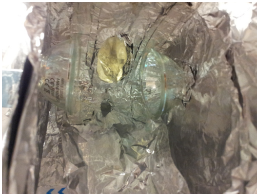
(a) Preform torn by hydrostatic pressure of GaIn during drawing of SEBS fibre
