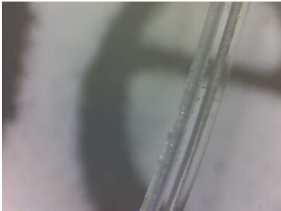
(e) Double channel fibre with GaIn in righthand channel
