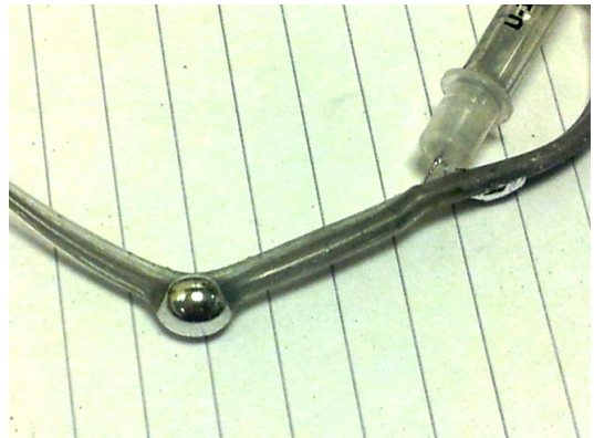
(d) GaIn 'aneurysm' preventing post drawing filling of hollow channelled SEBS fibre.
