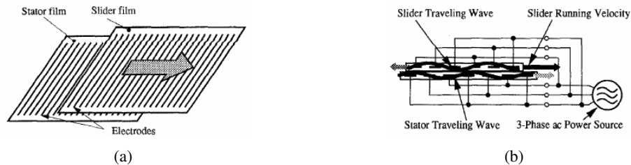
Figure 12-8: a) Schematic of Dual Excitation Multiphase Electrostatic Drive (DEMED). The electrodes are connected into three phases, fig-1 from [251]. b) Schematic cross sectional view of basic DEMED. Two potential distribution around electrodes are indicated by bold lines, fig-2 from [251].
