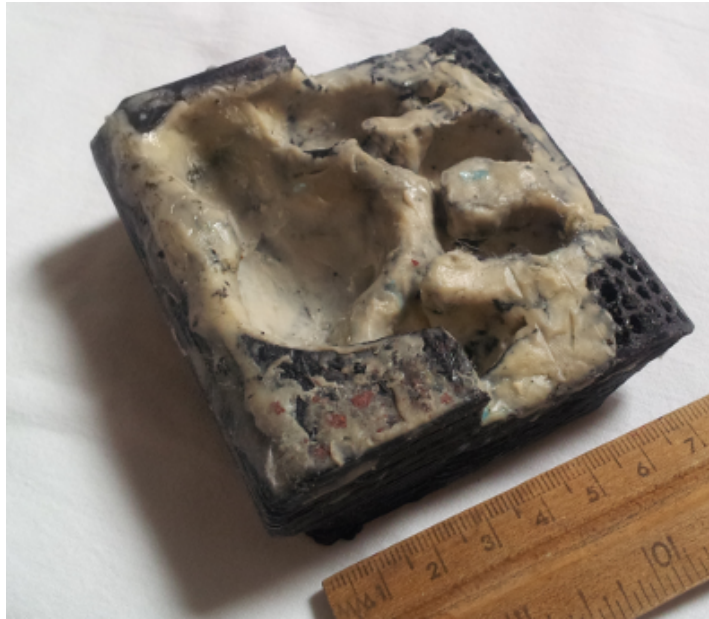
Figure 10-1: Paw pad mould, 3D printed PLA, lined with modelling wax as a releasing layer.
