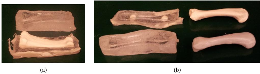
Figure 8-7: Polyurethane mould from anatomy skeleton bones to make polycaprolactone bones
