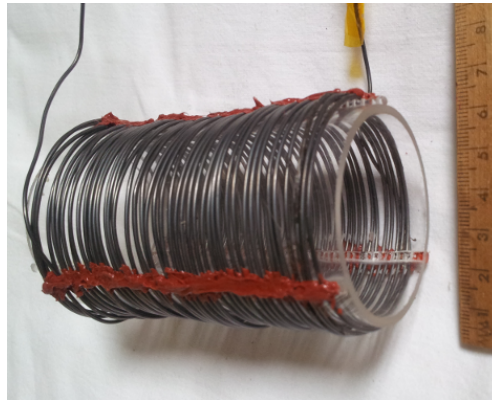
Figure 11-6: Cylindrical furnace, inner silica glass tube with nichrome resistor wire and high temperature silicone. The outer borosilicate glass tube is not shown.
