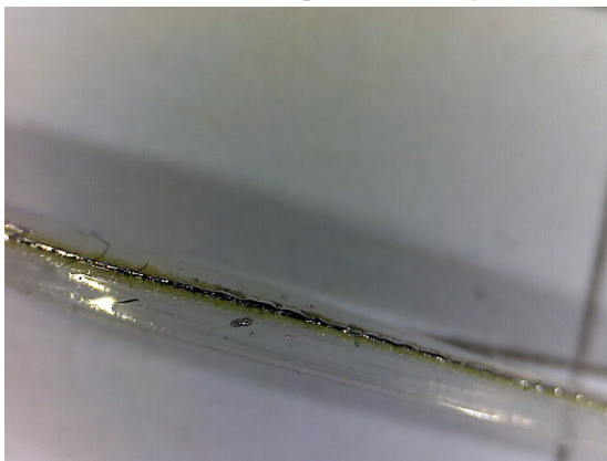
(c) Fibre EVA with micron-ITO (green) wetting agent
