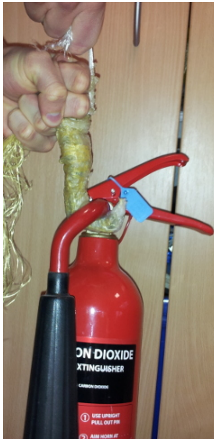
Figure 9-24: Demonstration of the strength of the finger as initially built. The flexor tendons were able to actuate the finger with force comparable to a human finger. Shown here lifting a fire extinguisher, approximately 5kg.
