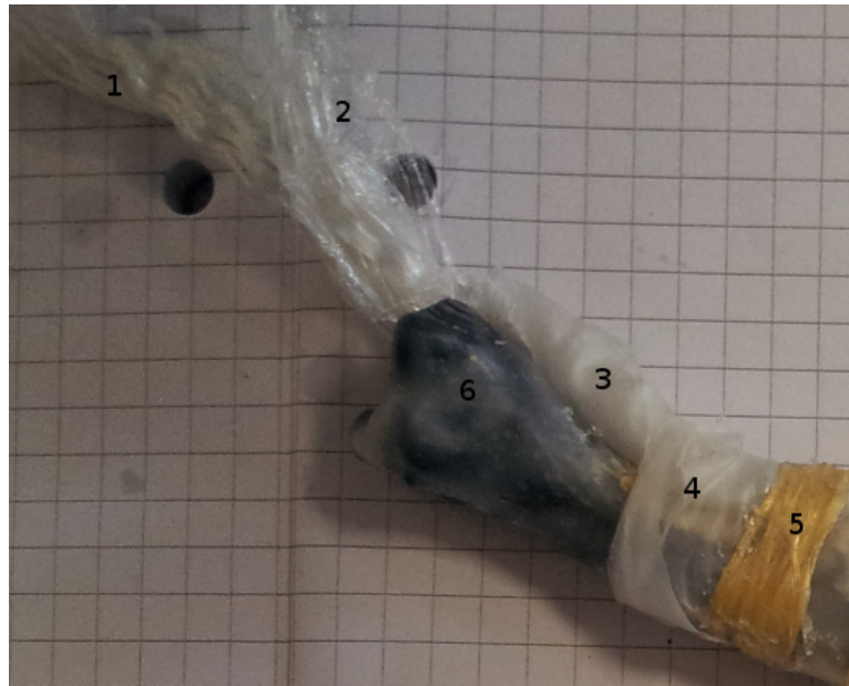
Figure 9-19: Structure of flexor sheath - (1)PA-66 tendons with SEBS-paraffin gel matrix, (2)MD-PE lining, (3)Elasto-5000 layers around sheath and as (4)matrix to annular ligaments, (5)polyaramide (PAr) tows of annular ligament, (6)PCL coated PLA bone.
