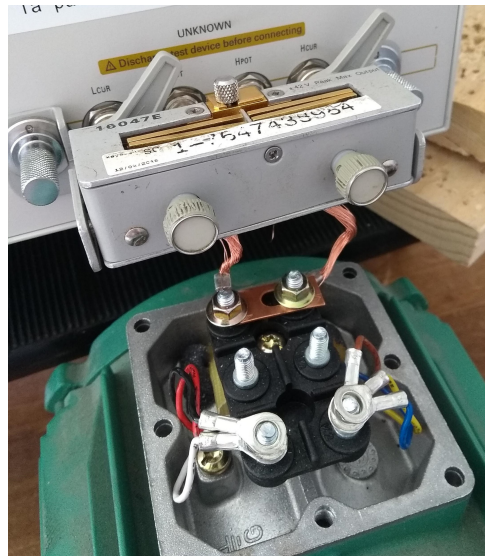
Figure H.3 – Motor input impedance measurement setup: compensation SHORT
