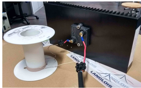
Figure 4.11 – The RL series load connected to the two-conductor 2.5\text{ mm}^2 cable
