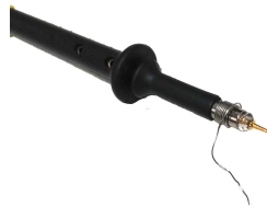
Figure 2.20 – Connection of the voltage probe along the line
