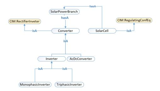
Figure 2.12: Extract of the Photovoltaic Branch package
