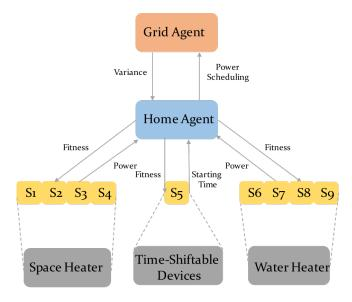
Figure 4.1: CPSO Configuration and Operation
