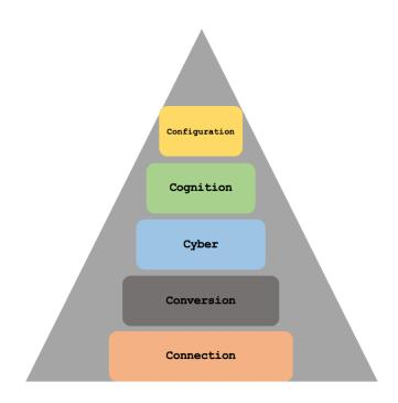
Figure 1.5: 5C Architecture for Cyber-Physical Systems
