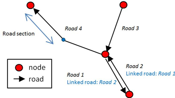
FIGURE 2.3 – Structure des routes et des intersections (Czura *et al.*, 2015).
