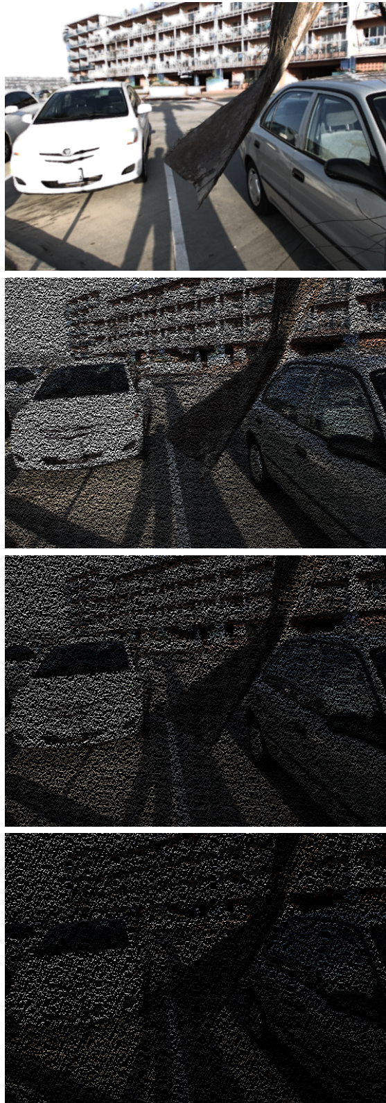
Figure 4.2: Examples of sampled images of the light field dataset Cars at different sampling rates. Top to bottom: original image, 40%-sampling, 20%-sampling and 10%-sampling.
