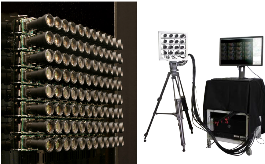
Figure 1.3: Example of camera array for light field capture: Left: Stanford multi-camera Array [12]. Right: Technicolor’s camera array [10] prototype, composed of 16 video cameras.
