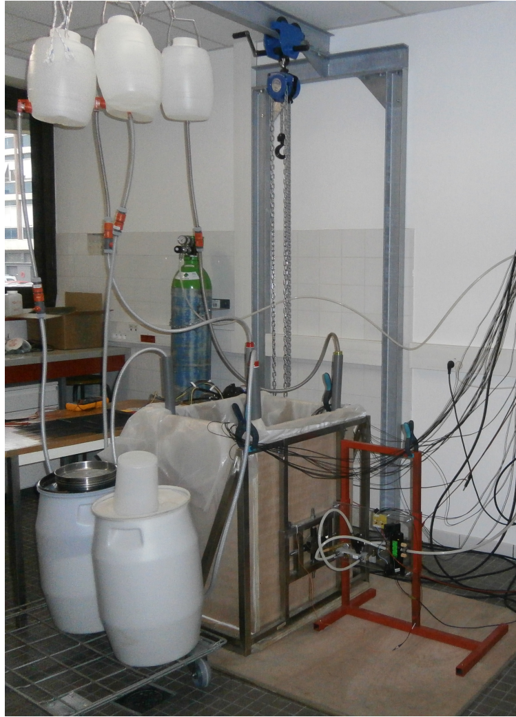
Figure 3.2: Global view of the sandbox, the pneumatic source and the water injection system.
