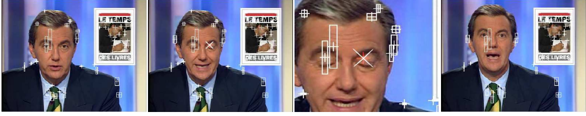
Figure 3.3: Categorization of interest points, according to their spatio-temporal behavior: the boxes represent the amplitude of moving points along their trajectory (motionless points do not have a box). The "+" corresponds to the mean position of such points. The "x" shows a non persistent point (the eye blinking).
