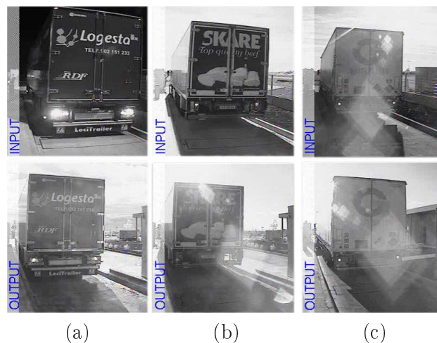
Figure 2.11: Three examples of successful recognition between truck arriving (first row) and leaving (second row). Here, license plate detection failed, because of: (a) plate saturated due to sidelight too strong; (b) and (c) very low sun and dirty plate.
