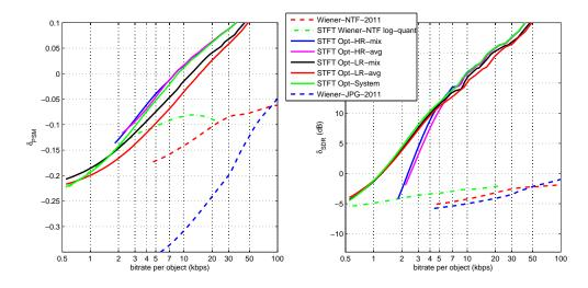
FIGURE 5.2 – CISS-NTF with different ways of optimizing parameters (solid lines), compared to state of the art  $[LPB^+12]$  (dotted lines).  $\delta PSM$  and  $\delta SDR$  denote the improvements over the corresponding measures computed for the oracle Wiener filtering [VGP07] source estimates in the STFT domain (figure from [3]).
