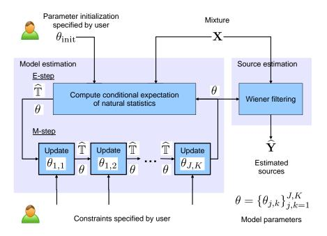
FIGURE 4.3 - Overview of the proposed general MU-GEM algorithm for parameter estimation and source separation (figure from [2]).
