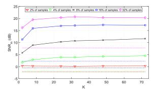
Fig. 5: The reconstruction performance measured in terms of  $SNR_m$  of a 4s long music signal from its random samples. The reconstruction results with our proposed algorithm (solid lines) are shown for different percentage of samples and different number of components, K, used in our approach. The results with shape preserving piecewise cubic interpolation are also shown for comparison (dashed lines), with the colors indicating corresponding percentage of samples.
