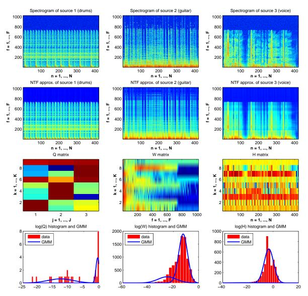
Fig. 5. Source MDCT power spectrograms  $p_{jfn}$  (5) (first row), their structured approximations  $v_{jfn}$  (3) (second row), NTF matrices (third row), histograms of NTF log-coefficients (*bars*) and two-state GMMs (*solid line*) modeling them (fourth row). In this example J = 3, F = 1024, N = 421 and K = 9.
