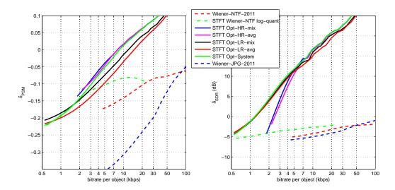
Fig. 6. CISS-NTF with STFT and different ways of optimizing parameters, compared to state of the art.  $\delta$ SDR and  $\delta$ PSM denote the improvements over the corresponding measures computed for the oracle Wiener filtering source estimates in the STFT domain.
