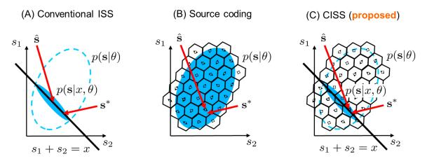
FIGURE 5.1 – Simplified visualization of the following probabilistic model-based methods applied in one TF point : (A) conventional ISS [LPB+12], (B) source coding and (C) the proposed coding-based ISS (CISS). Notations : x : mixture,  $\mathbf{s} = [s_1, s_2]^T$  : sources,  $p(\mathbf{s}|\theta)$  : *a priori* source distribution,  $p(\mathbf{s}|x,\theta)$  : *a posteriori* source distribution,  $\mathbf{s}^*$  : true sources,  $\hat{\mathbf{s}}$  : estimated sources.
