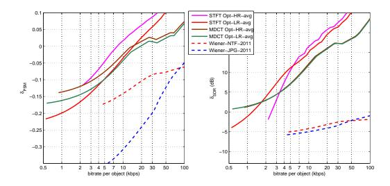
Fig. 7. CISS-NTF with MDCT and STFT vs. the state-of-the-art. Evaluation was performed using both STFT and MDCT transforms.  $\delta$ SDR and  $\delta$ PSM denote the improvements over the corresponding measures computed for the oracle Wiener filtering source estimates in the STFT domain.
