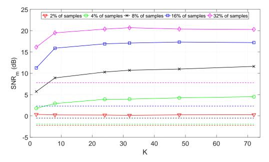
FIGURE 6.4 – The reconstruction performance measured in terms of  $\text{SNR}_m$  of a 4s long music signal from its random samples. The reconstruction results with our proposed algorithm (solid lines) are shown for different percentage of samples and different number of components, K, used in our approach. The results with shape preserving piecewise cubic interpolation are also shown for comparison (dashed lines), with the colors indicating corresponding percentage of samples (figure from [4]).
