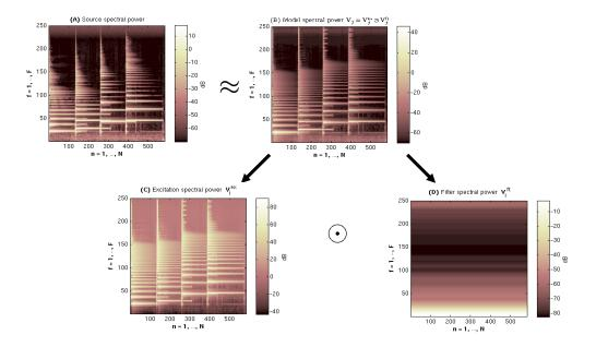
Fig. 3. Excitation-filter decomposition as applied to the spectral power of several guitar notes. (A): source spectral power, (B): model spectral power  $\mathbf{V}_j = \mathbf{V}_j^{\text{ex}} \odot \mathbf{V}_j^{\text{ft}}$ , (C): excitation spectral power  $\mathbf{V}_j^{\text{ex}}$ , (D): filter spectral power  $\mathbf{V}_j^{\text{ft}}$ .
