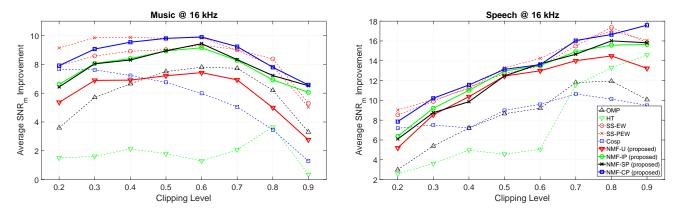
(a) Average  $SNR_m$  improvement computed over 10 music signals. (b) Average  $SNR_m$  improvement computed over 10 speech signals. Fig. 2: The average performance of all the audio declipping algorithms as a function of the clipping threshold (lower threshold corresponds to more severe clipping).
