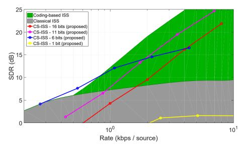
FIGURE 6.5 – The rate-distortion performance of CS-ISS using different quantization levels of the encoded samples. The performance of the ISS algorithm from  $[LPB^+12]$  and the coding-based ISS algorithm from [3] are also shown for comparison (figure from [4]).
