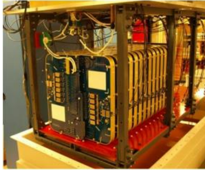
Figure 1. The Yale Marx 500 kV modulator charges many stages in parallel at low voltage, then discharges in series at high voltage. Each 12.5 kV, 250 A “flat pack” module is identical, providing for low fabrication and assembly cost.
