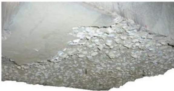
c) Heated face of the slab loaded at 15 MPa
