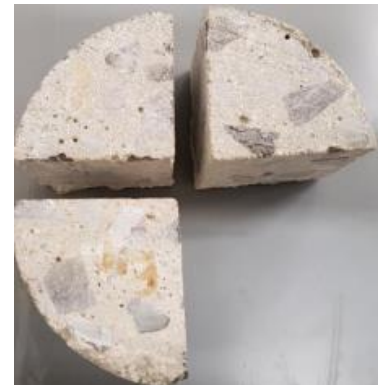
Water absorption porosity test specimens
