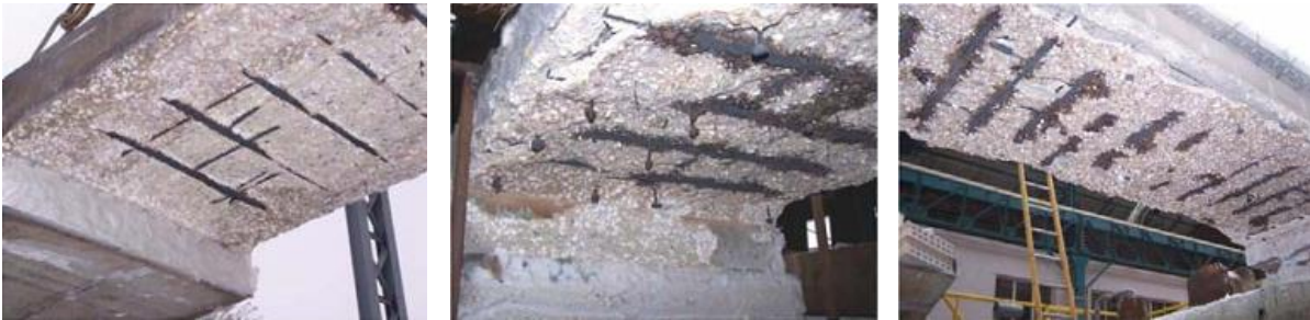
a) Thermal protection = 0 mm Maximum depth = 49 mm
