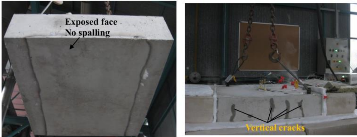
Figure 4.16: Exposed face (left); cracking and released of hot moisture (right) during the test.
