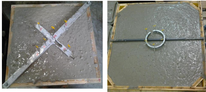
Figure 3.1: The images right after cast concrete from PT test (left) and biaxial fire test (right).
