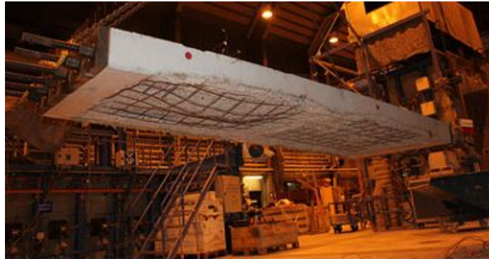
Figure 2.8: The test specimen after the fire exposure [29].
