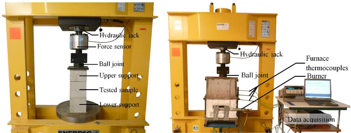
Figure 4.3: Tested sample in the hydraulic press (left) and complete test setup (right).
