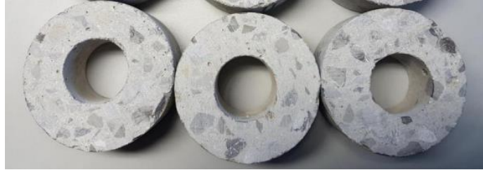
Figure 3.10: Radial permeability test specimens.
