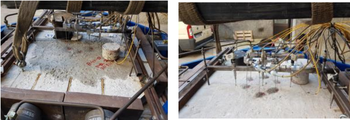
Figure 4.22: Released of hot moisture during the fire tests of B40-II in the unloaded (left) and loaded at 3 MPa (right).
