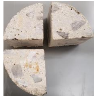
Water absorption porosity test specimens
