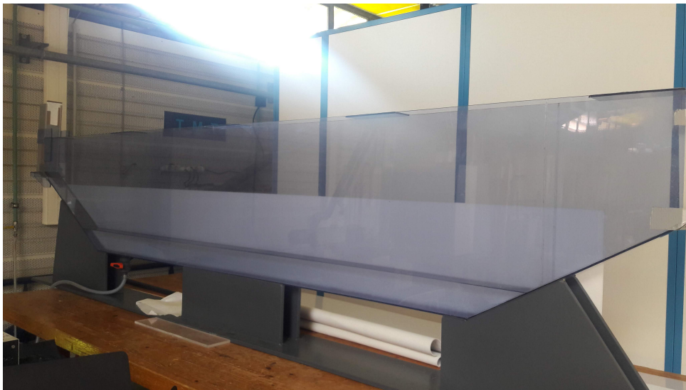
Figure 3.12: Picture of the experimental tank with two inclines and a reservoir on the left incline
