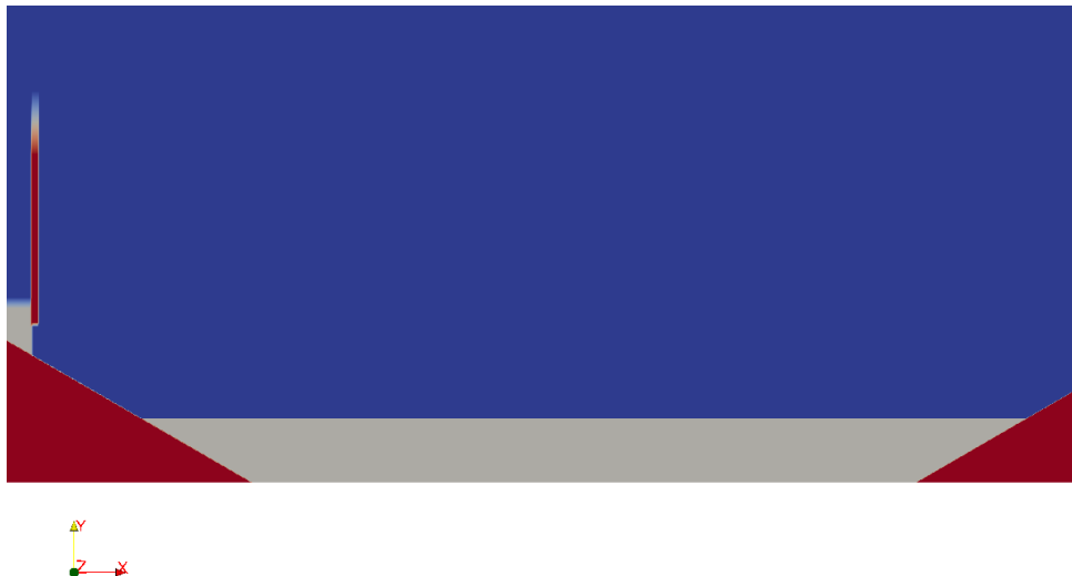
Figure 5.1: Picture of the numerical domain reproducing the experimental tank with two inclines and the reservoir
