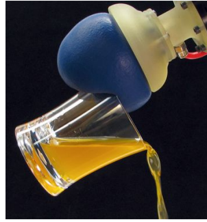
Figure 1.5: Universal soft gripper presented in (Brown et al. 2010).
