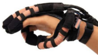
Figure 1.4: Soft robotic glove presented in (Polygerinos et al. 2015).
