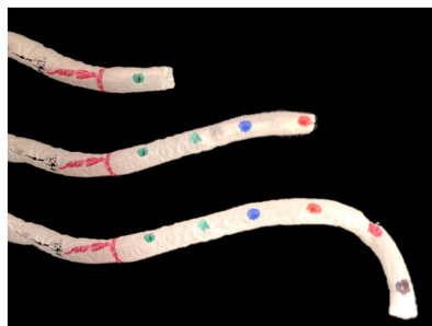
Figure 1.3: Growing robots used for catheter navigation in (Slade et al. 2017).
