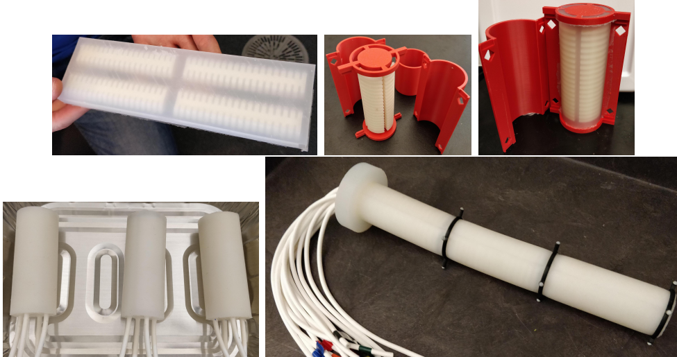
Figure 3.7: Manufacturing overview of the 3D soft arm. From Top Left to Bottom Right: Creation of four wax cores through casting; assembly of wax cores into 3D printed molds; casting of Silicone Rubber into the mold; Removal of wax through melting and addition of silicone tubing; Routing of tubing, gluing, labeling and adding markers.
