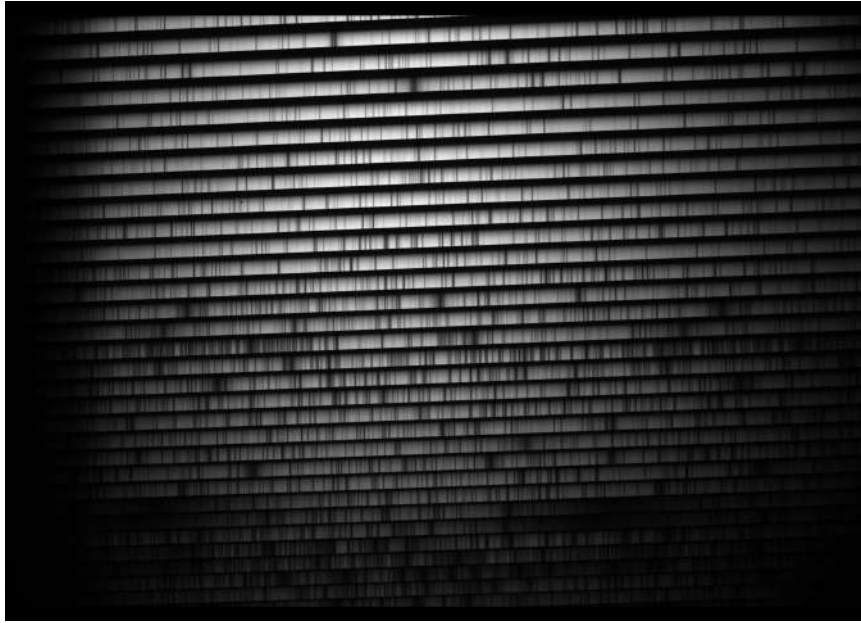
Figure 4.18: Example echelogramme showing the various spectral orders. Many Fraunhofer absorption lines are visible along the spectral orders.
