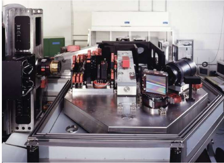
Figure 4.8: UVES spectrograph's test bench mount of its diverse elements (image: ESO's website ).
