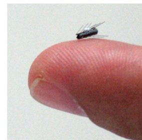
FIGURE 2 – Le micro-robot Virob.
