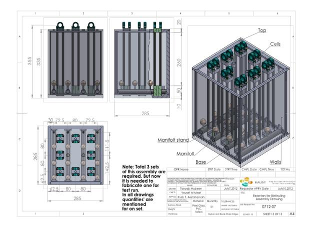
Figure G.1. Initial lab-scale MBR design.
