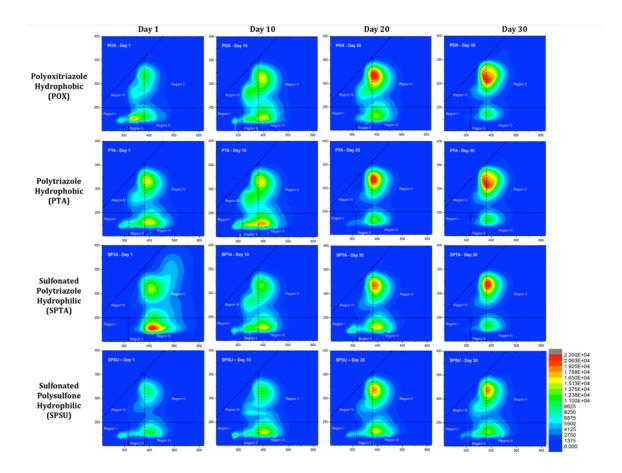
**Figure 4.10.** Evolution of 3D Fluorescence Excitation Emission (FEEM) diagrams for four different membranes operated with permeate production for 1, 10, 20 and 30 days.
