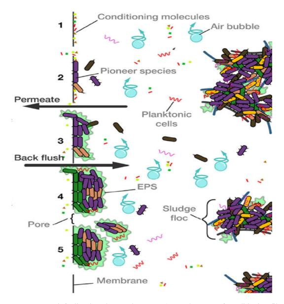
**Figure 1.8.** Biofouling in submerged MBRs: 1) Development of conditioning film; 2) Attachment of Pioneer microorganisms; 3) EPS production; 4) Development of microcolonies; 5) Detachment. (Adapted from Vanysacker et al. 2014) **[42]**.
