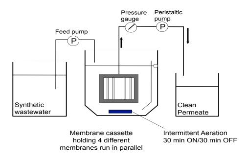
Figure 4.1. Schematic of the lab-scale membrane bioreactor (MBR).
