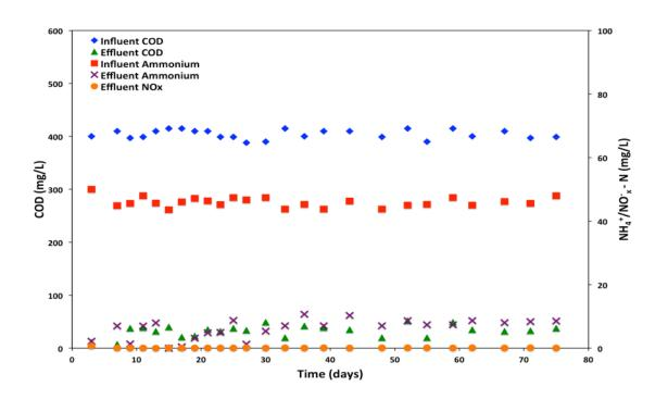
Figure 3.2. COD and ammonium concentrations in the synthetic wastewater influent and effluent, and nitrate  $(NO_3)$  and nitrite  $(NO_2)$  concentrations in the wastewater effluent.
