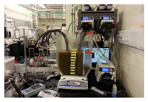
Figure G.3. Constructed lab-scale MBR in the Water Desalination and Reuse Center
