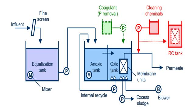
Figure 1.3. Universal MBR system configuration [2].
