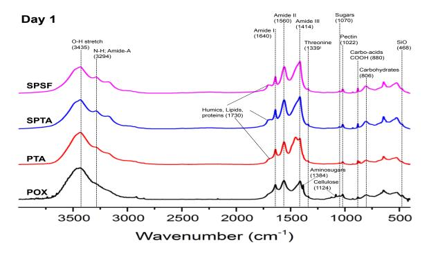
**Figure 4.3.** Fourier transform infrared (FTIR) spectroscopic analysis of the foulant material extracted from the four different membrane surfaces during early stages of filtration, operated with  $10 \text{ L/m}^2$ .h permeate production (1 day).
