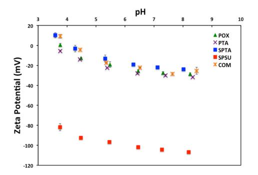
Figure C.3. Zeta potential measurements of the five clean membranes.
