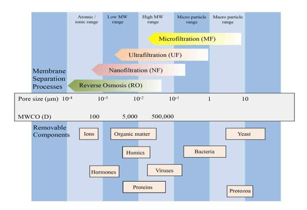
**Figure 1.2.** Membrane separation processes, pore size, molecular wright cut-off (MWCO) and examples of sizes of solutes and particles [5].
