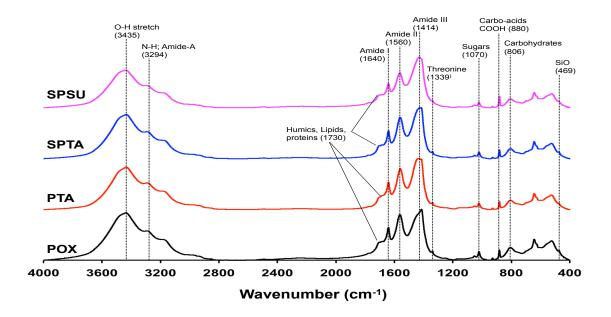
**Figure 4.4.** FTIR spectroscopic analysis of the foulant material extracted from the four different membrane surfaces inserted in the membrane tank, without permeate flux after 1 day of MBR operation.
