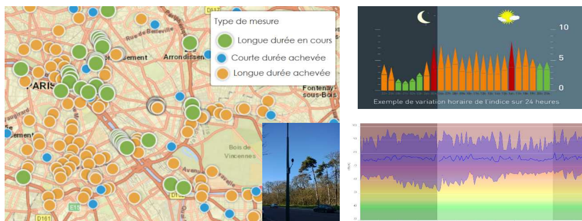
Figure 2:2 illustration of the RUMEUR network from BruitParif (website). Left: localization of the stations. Down: fixed measurement station from RUMEUR. Up right: Harmonica index. Down right: time series of LAeq,1s values available by clicking on a point of interest.
