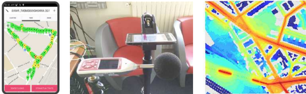
Figure 2:9 Illustration of the Ambiciti smartphone application. Left: screenshot of a measurement. Centre: calibration tests. Right: map from data assimilation. Source: (Ventura et al. , 2018).
