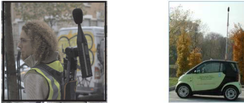
Figure 2:7 Illustration of the different mobile measurement methods. Left: mobile measurement ( Can et al., 2015 ). Right: mobile measurement point mounted on a mobile vehicle of the Sadmam network ( Manvell et al., 2004 ).
