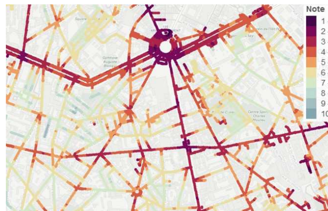
Figure 2:16 Example of sound pleasantness map interpolated from data collected through soundwalk. Source : Lavandier et al. , 2017 .
