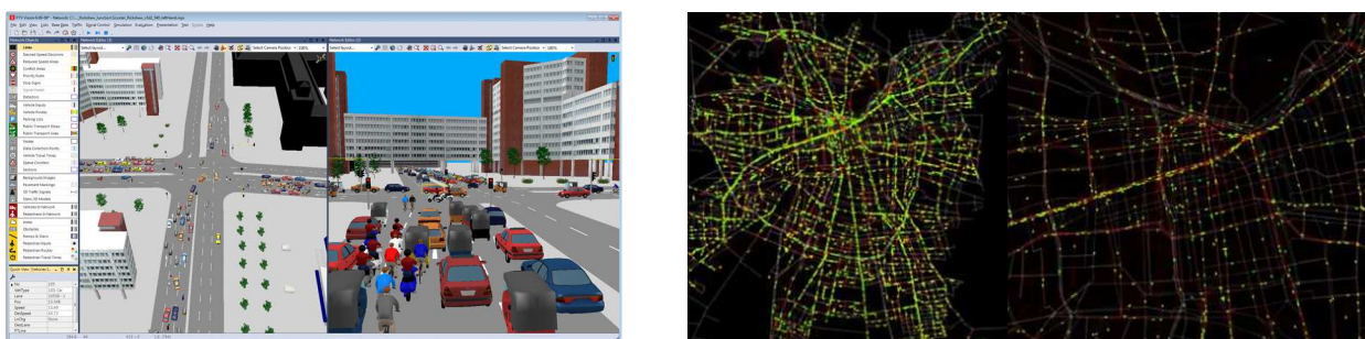
Figure 3:7 Illustration of two traffic software programs. On the left, VISSIM: the software aims to reproduce the trajectories and interactions between each vehicle (Source: PTV, 2011). On the right, MATSim: the objective of the model is to reproduce network and day-scale movements, according to individual activity patterns (Horni et al. , 2016).
