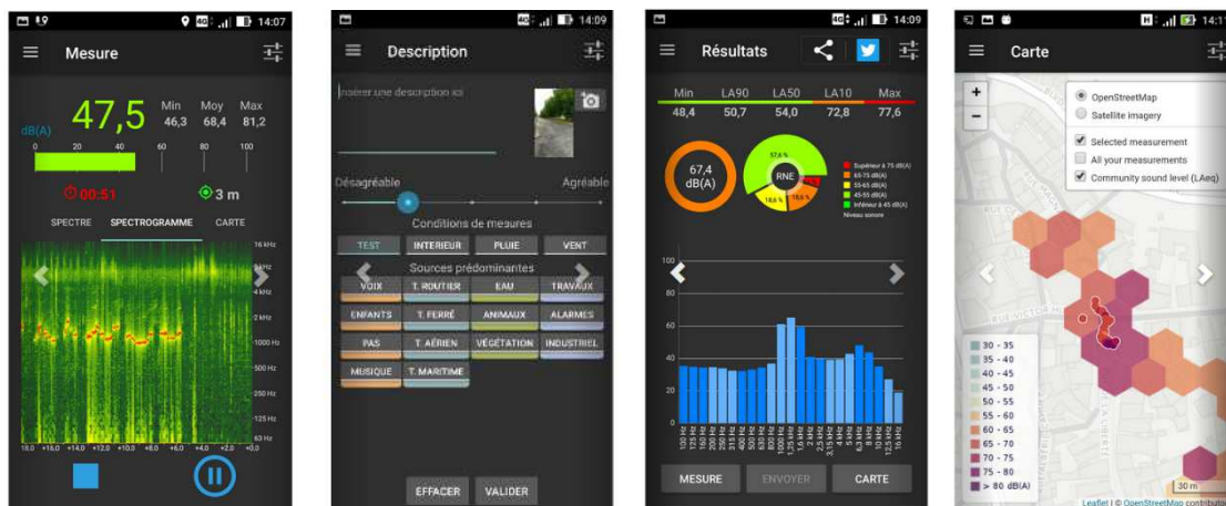
Figure 2:10 Illustration of the NoiseCapture smartphone application. From left to right: spectrogram measured in live, tag of sound sources heard, exposure during a journey, and noise map produced on the server that can be displayed on the user's smartphone ( http://noise-planet.org/noisecapture.html ).
