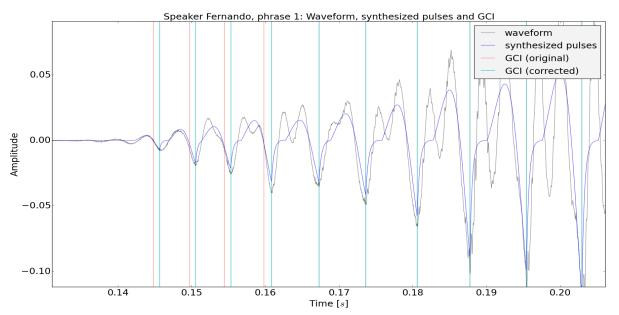
Figure 6.3: Speaker Fernando - Example of GCI timing correction
