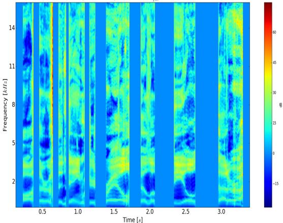
$\label{eq:time} \mbox{Time} \ [s] \\ \mbox{Figure 6.14: } \textit{Speaker BDL - Example of full-band VTF $C_{full}(\omega)$ without scaling to 0 dB mean}$ Speaker BDL, phrase 1: VTF  ${\cal C}_{\it full}$  - Full-band (zero mean)
