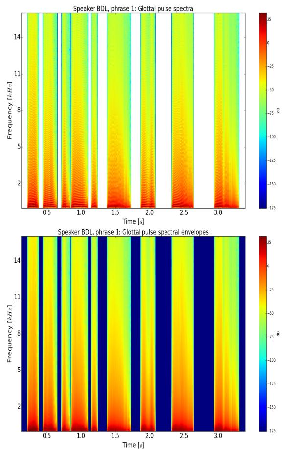
Figure 6.9: Speaker BDL - Spectra of glottal pulse  $g_s(n)$  and envelope  $\mathcal{T}_g$  sequence
