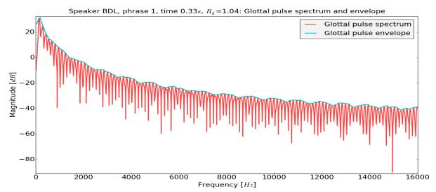
Figure 6.6: Speaker BDL - Glottal pulse spectrum  $G_s(\omega)$  and spectral envelope  $\mathcal{T}_g(\omega)$  example
