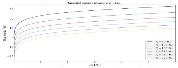
Figure 6.19: RMS-based energy contours  $E_{LF}$  of synthesized LF glottal pulses in dB
