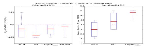
Figure 6.43: VQ Test 1 Speaker Fernando - Results for R<sub>d</sub> offset 0.0 with RMS energy scaling
