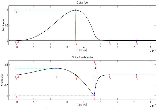
Figure 3.1: The glottal flow and its derivative in the time domain
