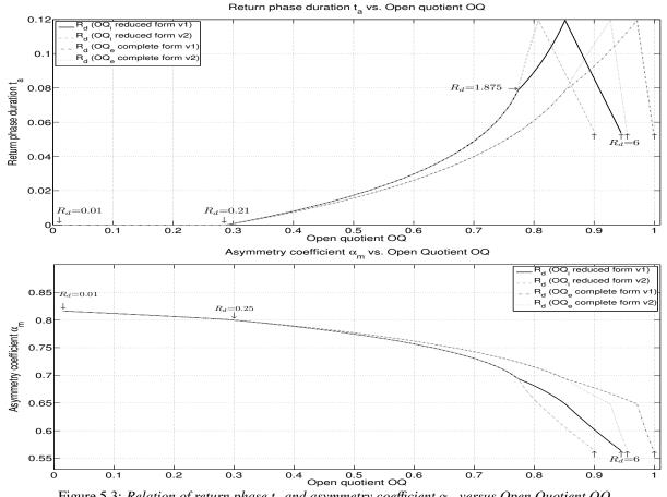
Figure 5.3: Relation of return phase  $t_a$  and asymmetry coefficient  $\alpha_m$  versus Open Quotient OQ
