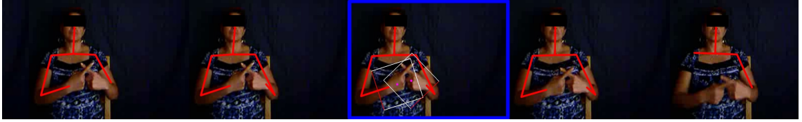
Figure 4.2 An illustration of proposed skeleton filtering in function. The frames are arranged from left to right with respect to their appearance in time. It can be observed that the output (frame with blue boundary) of our filtering strategy copes with the missing joint coordinates in the window. Gaussian smoothing is also applied on the joints which absorbs jitter in the raw output skeleton from openpose . The opted size of window is 7 frames, while only 5 frames are shown for clarity. The bounding boxes on the hands are extracted as a part of proposed spatial attention module detailed in Section 4.3.2
