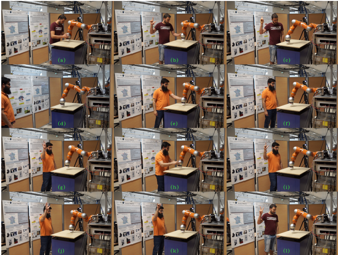
Figure 3.13 Screenshots from the robotic experiment by operators Op1 and Op2 (a) Op1 manually guiding the robot to a waypoint in the workspace. (b) Op1 records the way-points using Record gesture. (c) Op1 replay the taught waypoints by Replay gesture. (d) Op2 stands far from the robot so it moves with full speed. (e) Op2 stops the robot by applying external force (or accidental touch). (f) Op2 stands near the robot, so it moves slowly ensuring operator's safety. (g) Op2 gives Reteach command to the robot. (h) Op2 sets the new waypoints manually. (i) Op2 gives Record command. (j) Op2 stops the robot by Stop gesture. (k) Op2 resumes the robot operation by Resume gesture. (l) Op1 ends the robot operation by giving End command.
