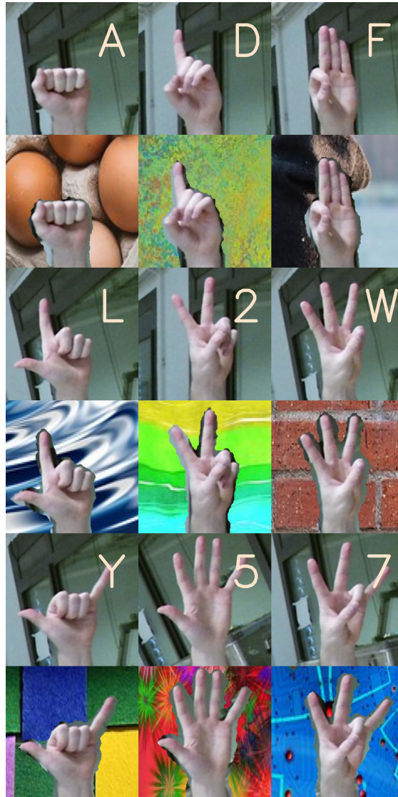
Figure 3.6 Samples of hand gesture images with original (labeled images) and substituted backgrounds (below originals). Note the remnants of the original backgrounds. This phenomenon is due to dilation of the binary masks. While it could be avoided by using techniques like chroma key, we do not intend to use a uniform background, to avoid bringing any extra apparatus in operation. In the experimental results (Sect. 3.3.4), we show that despite these remnants, gesture detection is highly accurate.
