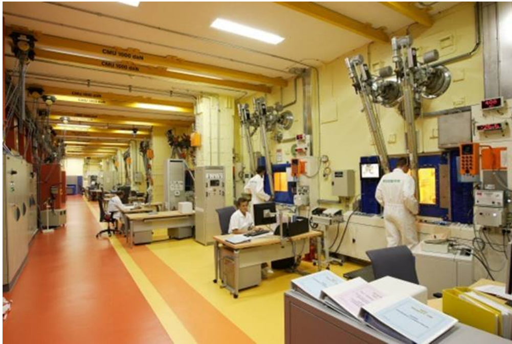
Figure 1.2: Hot cells and teleoperation zone
