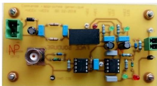
Fig. 3-18. Gate driver circuit.
