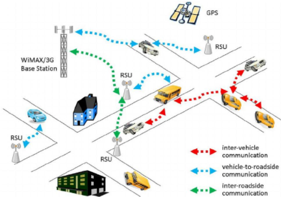
Fig. 2.4 Example of hybrid V2X communications in VANETs [56]
