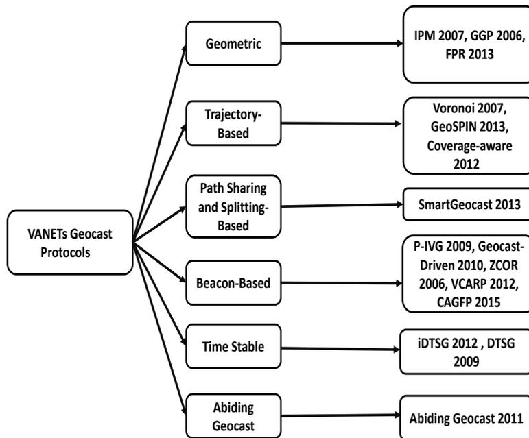
Fig. 2.9 Categories of geocast protocols in VANETs
