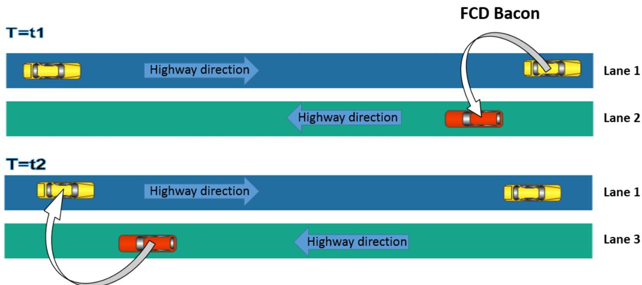
Fig. 4.3 FCD message propagation on a bidirectional road
