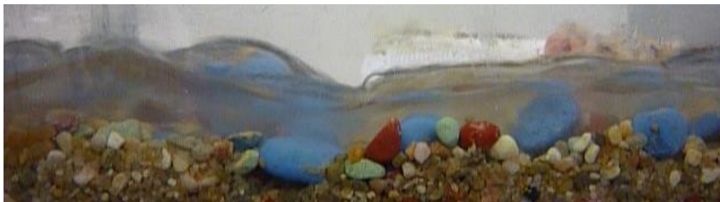
Figure 11 : Shallow flow over a non uniform grain size distribution in a flume
