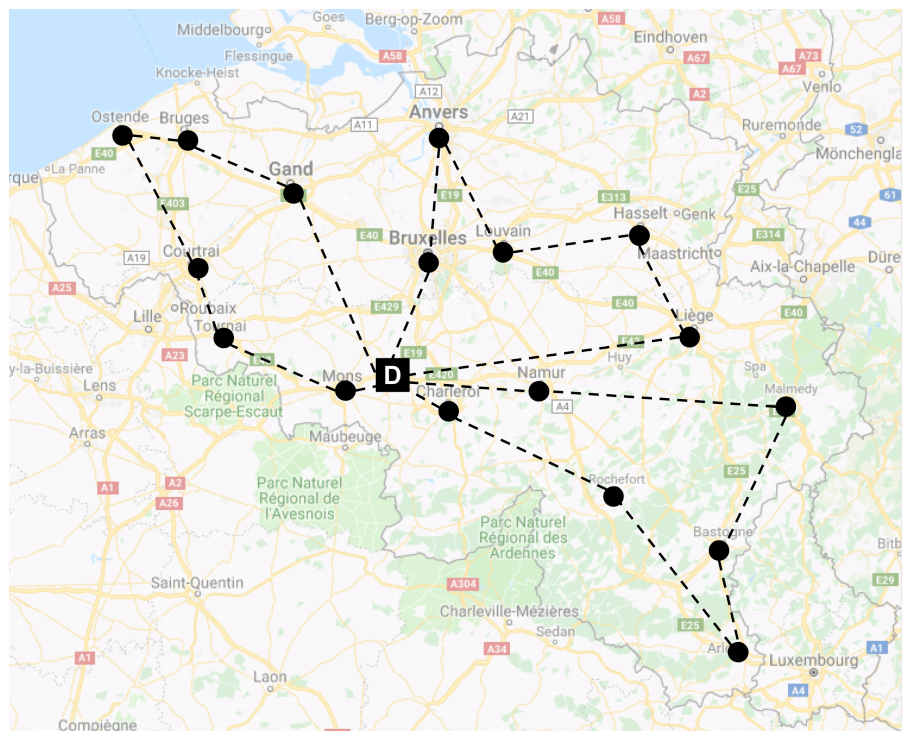
Figure 1.2: A possibly optimal solution to our Belgium VRP problem. We assume customer unit demands. Our depot is located in La Louvière and hosts at least three vehicles, each of maximal capacity of six.
