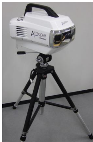
Figure 1-6 : Le corps de la caméra gamma ASTROCAM 7000HS (TAKEDA & al., 2015).
