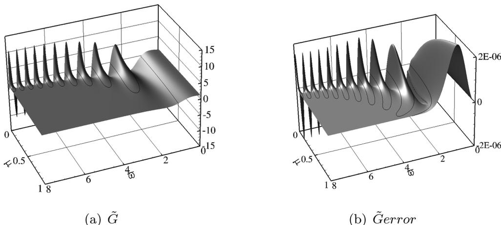
Fig. 2. Results for the evaluation of  $\tilde{G}$  with the ODE and error with the direct integration method. The ODE is solved using the RK4 method with  $\Delta\varpi = 0.001$   $\varpi \in (0, 8]$ , and  $\mu \in [0, 1)$ .
