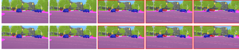
Figure 4.4: From left to right: two input frames and three predictions, framed in red, obtained from the warping baselines, “ t + 1 - centric” (top) and “ t - centric” (bottom). Static pixels that are about to be occluded by the moving objects are systematically mis-predicted to hold their previous values in the original baseline - see the pixels in front of the left car on the top row - leading moving objects to shrink instead of moving. This is corrected in our improved baseline, shown in the bottom row.
