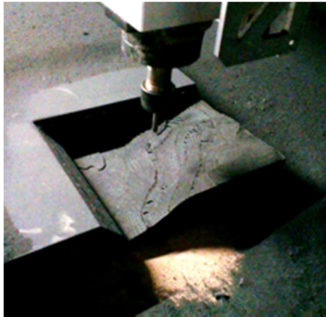
Figure 6. A first attempt on carving the map with a CNC machine on MDF
