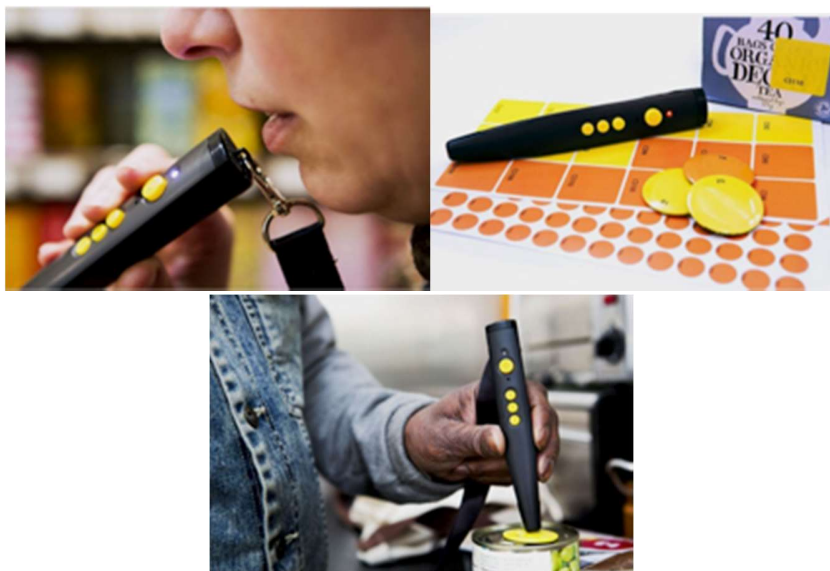
Figure 10. The usage of a Penfriend to identify objects.
