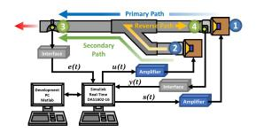
Fig. 2. Duct active noise control test-bench diagram.
