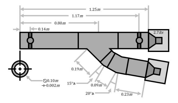
Figure 4: Duct active noise control test bench dimensions.
