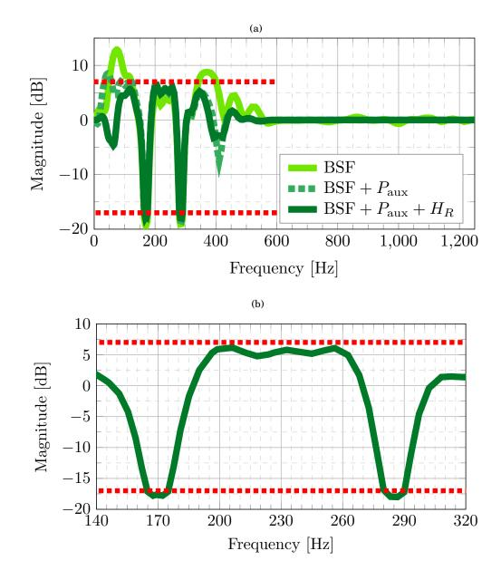
FIGURE 5.4. Output sensitivity function  $S_{yp}$ : a) Evolution of the fixed robust controller, and b) final controller zoomed region of interest.
