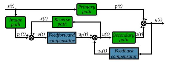
FIGURE 2.2. Block diagram representation of the combined feedback and feedforward control problem. In green we can identify the blocks corresponding to the system's plant, meanwhile in blue the corresponding  $feedback\ K$  and  $feedforward\ N$  compensators.
