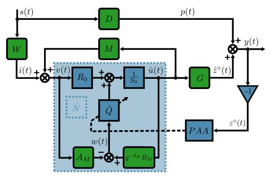
FIGURE 6.10. Feedforward control scheme using a Youla-Kučera parametrization with PAA.
