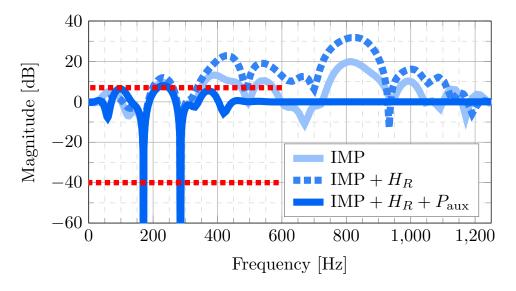
Figure 5.3. Evolution of the Output sensitivity function  $S_{yp}$  of a fixed linear controller.
