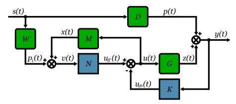
FIGURE 2.4. Block scheme of the combined feedback and feedforward control problem.
