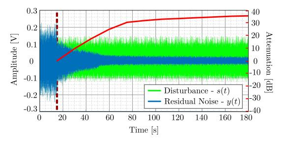
FIGURE 6.16. Performance of YK-IIR compensator order 30/30 with FuSBA PAA and constant trace profile (tr[F] $_{pp}$  = 0.10). Right side shows the level of attenuation achieved at a given point in time, with 35.6 dB achieved at 180 s. Compensation starts at 15 s.
