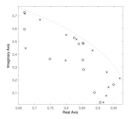
Figure 9: Zoom for the comparison of the positive feedback loop poles when using YKFIR ( $\circ$ ) and FIR ( $\times$ ) adaptive compensators (simulation).
