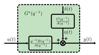
FIGURE 4.1. ARMAX process diagram.
