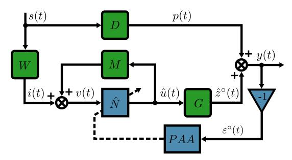
FIGURE 6.9. Feedforward control scheme with PAA.
