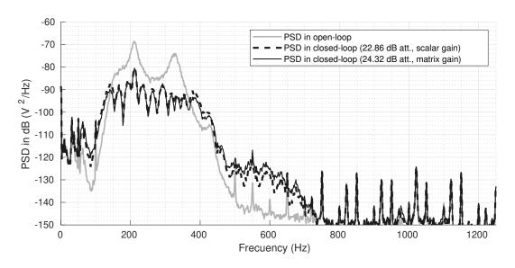
Figure B.16: PSD estimate of the YKFIR 60/0 adaptation compensator with scalar and matrix adaptation gains (constant trace of 60).
