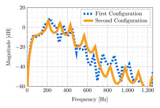
FIGURE 6.3. Identified secondary path for first and second test bench configurations.
