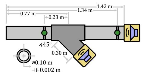
FIGURE 3.11. Third experimental test bench configuration.
