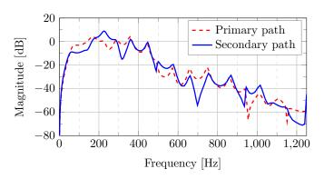
Fig. 7: Frequency characteristics of the identified primary and secondary paths models
