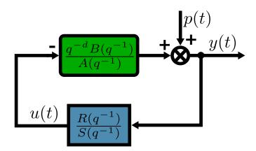
FIGURE 5.1. Feedback regulation scheme.
