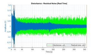
Fig. 20. Residual noise of the FIRYK 60/0 adaptive feedforward compensator for a change of disturbance from 170 - 270 Hz to 70 - 170 Hz at 180 s.
