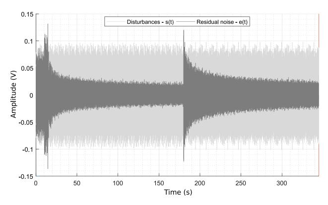
Figure 11: Transient performance of YKFIR adaptive compensator (experimental). 0 to 180s: broad-band disturbance 150-250 Hz; 180 to 345 s: broad-band disturbance 250-350 Hz; open loop operation: 0 to 15 sec.
