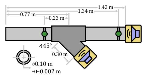
FIGURE 6.5. Third experimental test bench configuration.
