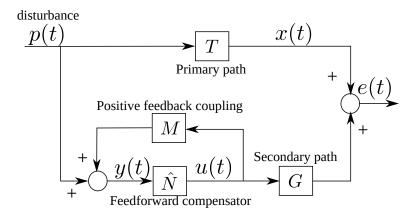
Figure 1: Adaptive active noise feedforward compensation.
