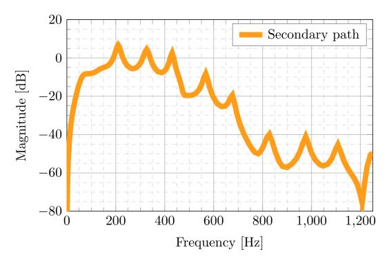
FIGURE 3.10. Second test bench configuration's identified secondary path.
