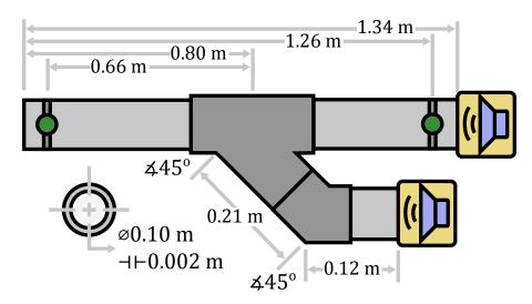
FIGURE 3.2. First experimental test bench configuration.
