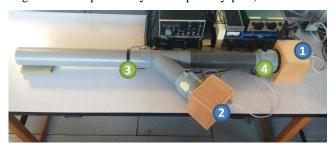
Fig. 3. Duct active noise control test-bench. Configuration A (Photo).
