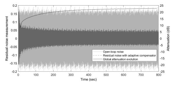
Figure B.15: Residual noise of the YKFIR 60/0 adaptation compensator with scalar gain (constant trace of 60, gain per parameter: 1).
