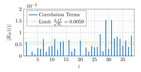
FIGURE 4.4. Whiteness test for identified secondary path.
