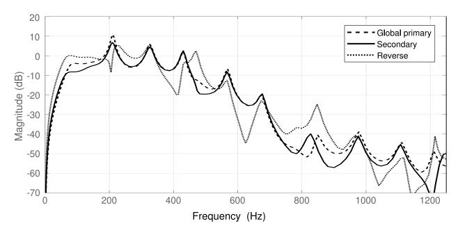
Figure 5: Frequency characteristics of the Primary, Secondary and Reverse paths identified models.
