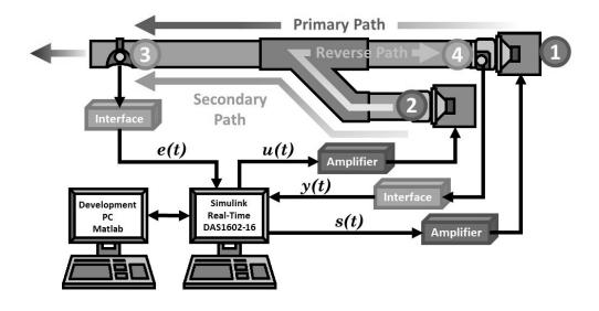
Figure 3: Duct active noise control test bench diagram.
