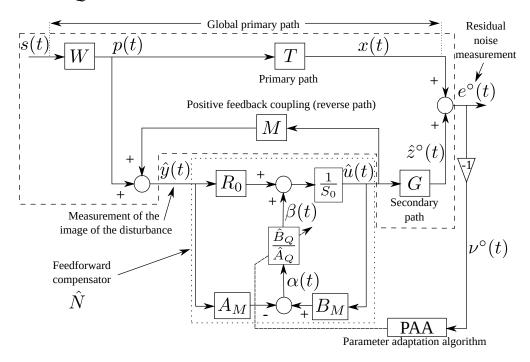
Figure 7: Adaptive feedforward disturbance compensation using Youla-Kučera parametrization.
