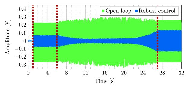
FIGURE 5.12. Residual noise in open loop vs closed loop using a robust controller under the effect of tonal disturbances with variable frequencies.
