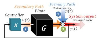
Fig. 3. Feedback regulation scheme.
