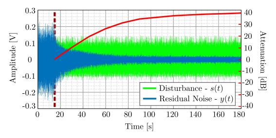
FIGURE 6.12. Performance of IIR compensator of order [15/15] with FuSBA PAA and constant trace profile ( $\text{tr}[F]_{pp} = 0.010$ ). Right side shows the level of attenuation achieved at a given point in time, with 39.6 dB achieved at 180 s. Compensation starts at 15 s.
