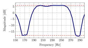
Fig. 6. Robust controller's output sensitivity function evolution—zoomed-in view.
