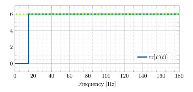
FIGURE 6.19. Evolution of adaptation matrix F's trace for a constant trace profile of a YK FuSBA PAA. A value of  $\text{tr}[F]_{pp}=0.10$  was chosen, so tr[F(t)]=tr[F]=6.0
