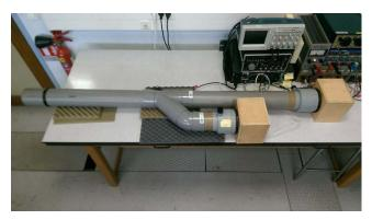
Fig. 1. Duct ANC test bench (photograph).
