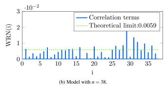
Fig. 5: Whiteness validation tests for the secondary path.
