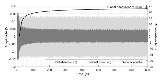
Figure 10: Performance of YKFIR adaptive compensator with 60 parameters (experimental).
