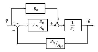
Figure 8: Equivalent representation of the Youla Kučera compensator.
