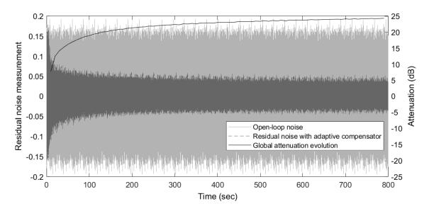
Figure B.14: Time domain evolution of the residual noise for the YKFIR 60/0 simplified adaptative compensator with matrix adaptation gain (constant trace of 60).
