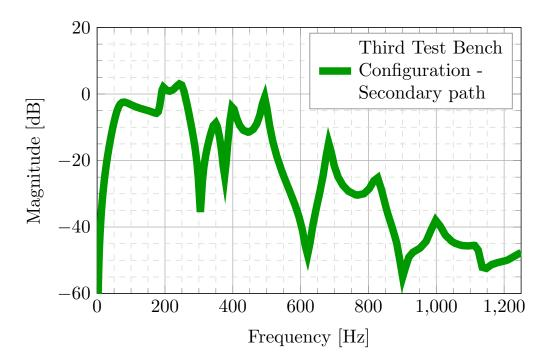
FIGURE 6.11. Identified secondary path for the third test bench configuration.
