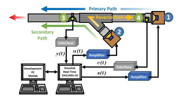
FIGURE 6.4. Schema of test bench's feedforward configuration.
