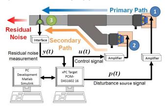
Fig. 2. Duct ANC test bench diagram.
