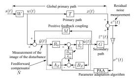
Fig. 2. Adaptive feedforward disturbance compensation using the generalized Youla-Kučera parametrization.
