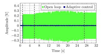
Fig. 12. Residual noise in open loop (green) and closed loop (blue) using an adaptive controller under the effect of tonal disturbances with variable frequencies.
