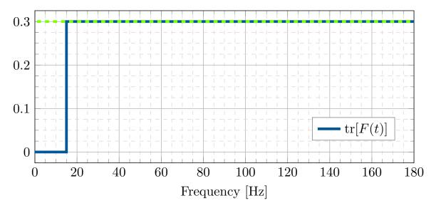
FIGURE 6.15. Evolution of adaptation matrix F's trace for a constant trace profile of a FuSBA PAA. A value of  $\text{tr}[F]_{pp}=0.010$  was chosen, so tr[F(t)]=tr[F]=0.3
