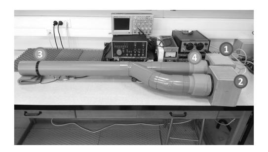
Figure 2: Duct active noise control test bench (Photo).
