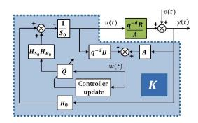
Fig. 7. Adaptive YK parameterization scheme.
