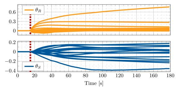
FIGURE 6.14. Filter  $N(q^{-1}) = \frac{R}{S}$  parameters evolution for a [15/15] standard IIR filter using FuSBA PAA with a constant trace profile. Compensation starts at 15 s.
