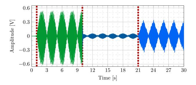
FIGURE 5.6. Acoustic interference attenuation using a robust controller.
