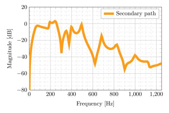
FIGURE 3.13. Third test bench configuration's identified secondary path.
