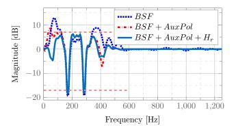
Fig. 5. Robust controller design: Output sensitivity function.
