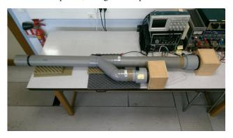
Fig. 1: Noise control test bench (Photo).
