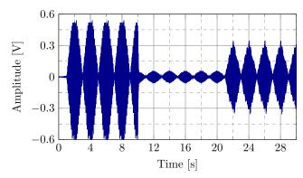
Fig. 8. Acoustic interference attenuation using a robust controller. Noise frequencies: 170 + 170.5 Hz and 285 + 285.5 Hz then 180 + 180.5 Hz and 295 + 295.5 Hz. Loop closed at 10 s.
