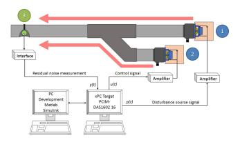
Fig. 2: Noise control test bench diagram.
