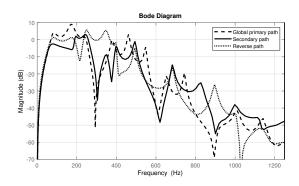
Fig. 4. Frequency characteristics of the Primary, Secondary and Reverse paths identified models.
