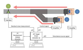
Fig. 1. Active noise control test bench diagram.
