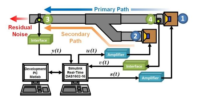
FIGURE 3.4. Schema of test bench's first configuration.
