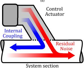
FIGURE 3.1. (a) Standard control actuator positioning. (b) Proposed control actuator positioning.
