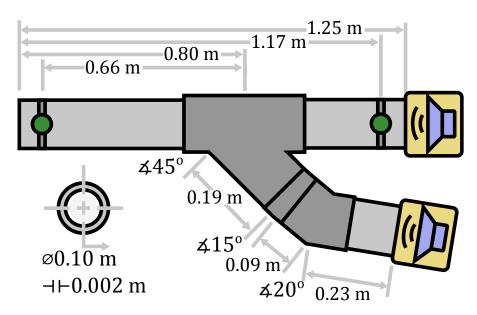
FIGURE 6.1. Second experimental test bench configuration.
