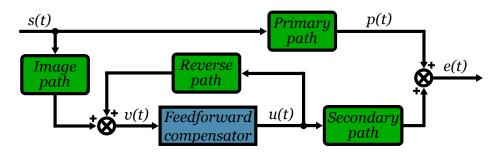
FIGURE 2.8. Feedforward control problem schema.
