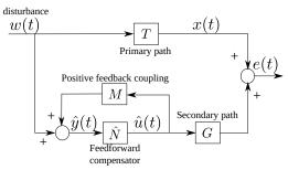
Fig. 1. Adaptive active noise feedforward compensation.
