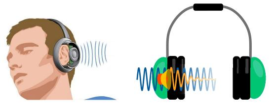
FIGURE 2.1. External noise attenuation in headphones by use of Active Noise Control.
