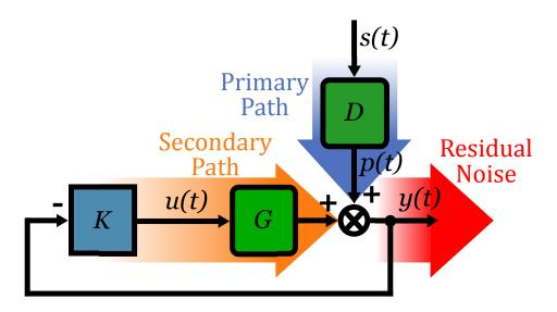
FIGURE 3.6. Feedback control scheme.
