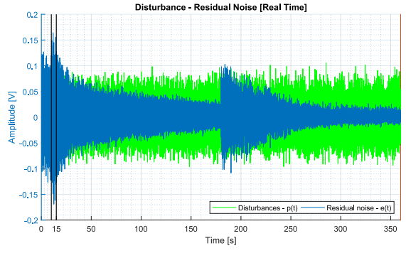
Fig. 11. Residual noise of the IIR 15/15 adaptive feedforward compensator for a change of disturbance from 170 - 270 Hz to 70 - 170 Hz at 180 s.
