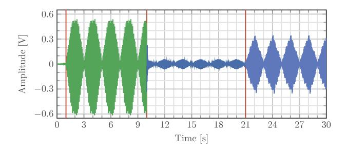
FIGURE 4.6. Acoustic interference attenuation using a robust controller.
