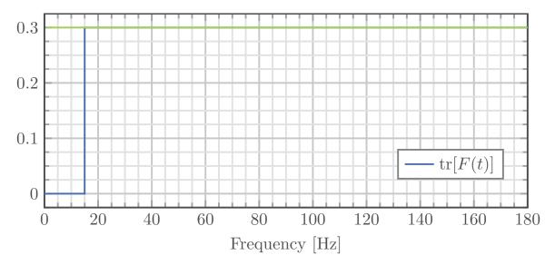
FIGURE 5.15. Evolution of adaptation matrix F's trace for a constant trace profile of a FuSBA PAA. A value of  $\text{tr}[F]_{pp}=0.010$  was chosen, so tr[F(t)]=tr[F]=0.3
