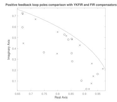
Figure 9: Comparison of the positive feedback loop poles for the YK FIR  $(\circ)$  and FIR  $(\times)$  adaptive compensators (simulation).
