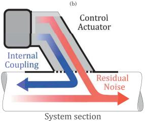
FIGURE 2.1. (a) Standard control actuator positioning. (b) Proposed control actuator positioning.
