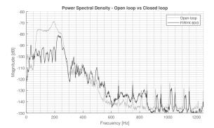
Fig. 18. PSD of the FIRYK 60/0 adaptive compensators using FUSBA matrix adaptation (70-270 Hz disturbance, 600 s experiments).
