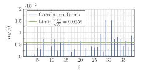
FIGURE 3.4. Whiteness test for identified secondary path.
