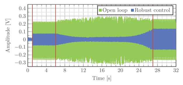
FIGURE 4.12. Residual noise in open loop vs closed loop using a robust controller under the effect of tonal disturbances with variable frequencies.
