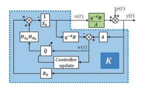
Fig. 7. Adaptive YK parameterization scheme.
