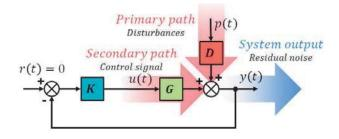
Fig. 3: Feedback regulation scheme.
