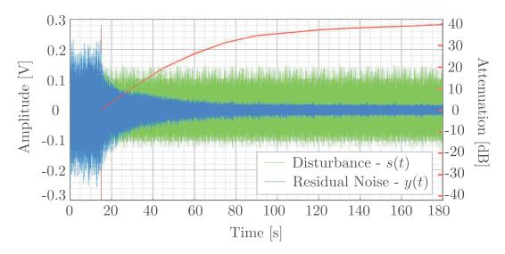
FIGURE 5.12. Performance of IIR compensator of order [15/15] with FuSBA PAA and constant trace profile ( $\text{tr}[F]_{pp} = 0.010$ ). Right side shows the level of attenuation achieved at a given point in time, with 39.6 dB achieved at 180 s. Compensation starts at 15 s.
