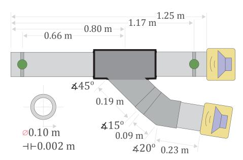
FIGURE 5.1. Second experimental test bench configuration.
