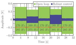
Fig. 14. Step changes in frequencies using the robust controller. Residual noise in open loop (green) and in closed loop (blue).
