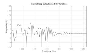
Fig. 19. Internal loop output sensitivity function for the FIRYK 60/0 adaptive compensator (70-270 Hz disturbance, 600 s experiments).
