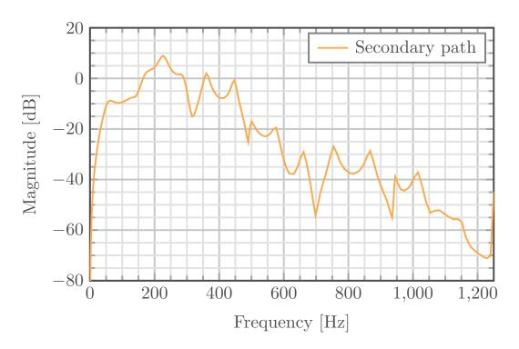
FIGURE 2.7. First test bench configuration's identified secondary path.
