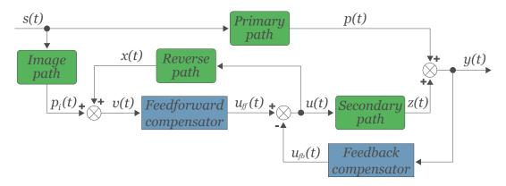
FIGURE 1.2. Block diagram representation of the combined feedback and feedforward control problem. In green we can identify the blocks corresponding to the system's plant, meanwhile in blue the corresponding  $feedback\ K$  and  $feedforward\ N$  compensators.
