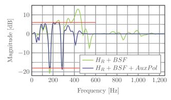
Fig. 5. Robust controller design—output sensitivity function evolution.
