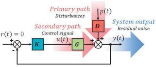
Fig. 3. Feedback regulation scheme.
