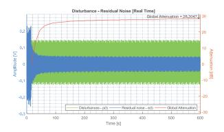
Fig. 16. Residual noise using the FIRYK 60/0 adaptive compensators with FUSBA matrix adaptation (70-270 Hz disturbance, 600 s experiments).
