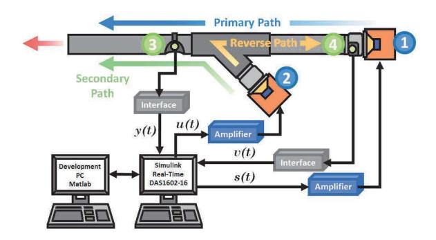
FIGURE 5.4. Schema of test bench's feedforward configuration.
