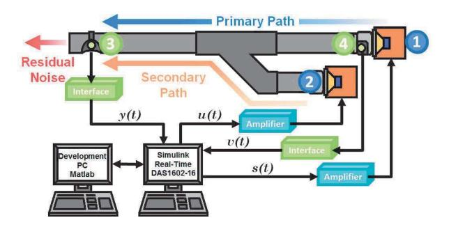
FIGURE 2.4. Schema of test bench's first configuration.
