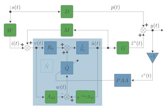
FIGURE 5.10. Feedforward control scheme using a Youla-Kučera parametrization with PAA.
