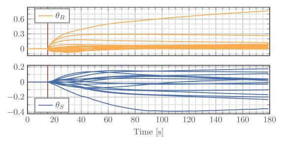
FIGURE 5.14. Filter  $N(q^{-1}) = \frac{R}{S}$  parameters evolution for a [15/15] standard IIR filter using FuSBA PAA with a constant trace profile. Compensation starts at 15 s.
