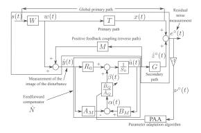
Fig. 6. Adaptive feedforward disturbance compensation using Youla-Kučera parametrization.
