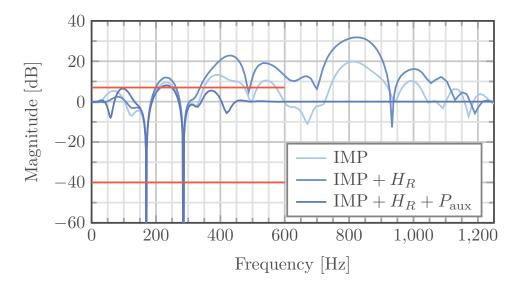
FIGURE 4.3. Evolution of the Output sensitivity function  $S_{yp}$  of a fixed linear controller.
