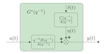
FIGURE 3.1. ARMAX process diagram.
