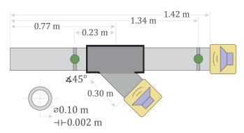
Fig. 3. Duct active noise control test-bench dimensions.
