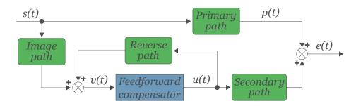
FIGURE 1.8. Feedforward control problem schema.
