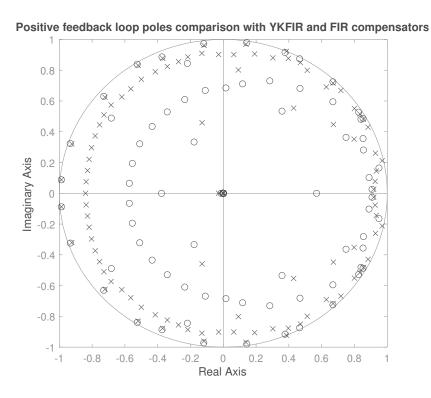
Figure 8: Comparison of the positive feedback loop poles for the YK FIR  $(\circ)$  and FIR  $(\times)$  adaptive compensators (simulation).
