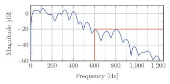
Fig. 9: Frequency characteristics for Input sensitivity,  $S_{up}$ .
