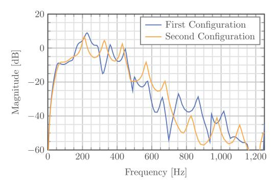
FIGURE 5.3. Identified secondary path for first and second test bench configurations.
