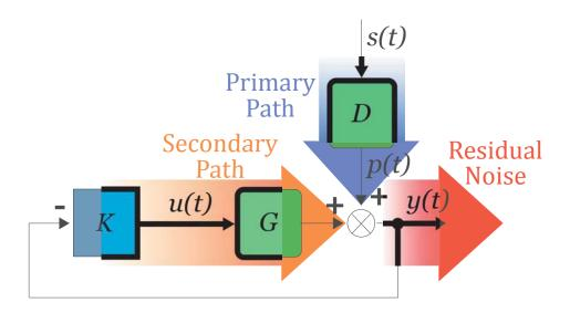
FIGURE 2.6. Feedback control scheme.
