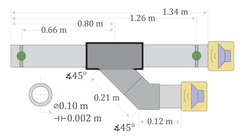
FIGURE 2.2. First experimental test bench configuration.
