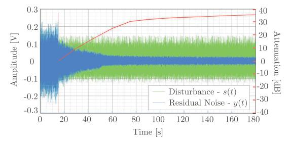
FIGURE 5.16. Performance of YK-IIR compensator order 30/30 with FuSBA PAA and constant trace profile (tr[F] $_{pp}$  = 0.10). Right side shows the level of attenuation achieved at a given point in time, with 35.6 dB achieved at 180 s. Compensation starts at 15 s.
