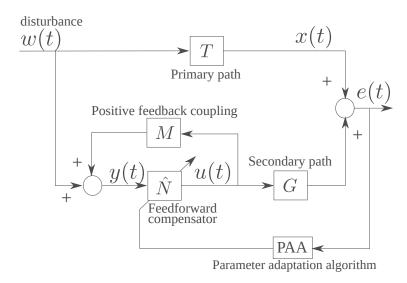
Figure 1: Adaptive active noise feedforward compensation.
