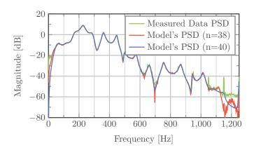
Fig. 6: System output PSD.
