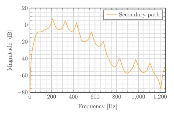
FIGURE 2.10. Second test bench configuration's identified secondary path.
