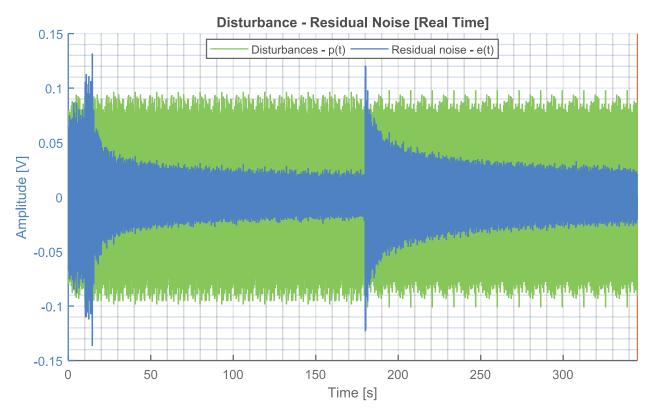
Figure 11: Transient performance of YK FIR adaptive compensator (experimental). 0 to 180s: broad-band disturbance 150-250 Hz; 180-345 s: broad-band disturbance 250-350 Hz; open loop operation: 0 to 15s
