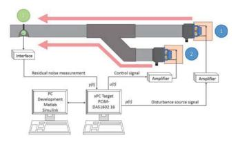
Fig. 2: Noise control test bench diagram.
