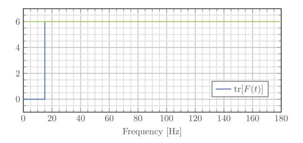
FIGURE 5.19. Evolution of adaptation matrix F's trace for a constant trace profile of a YK FuSBA PAA. A value of  $\text{tr}[F]_{pp}=0.10$  was chosen, so tr[F(t)]=tr[F]=6.0
