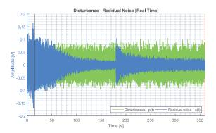
Fig. 15. Residual noise of the IIRYK 30/30 adaptive feedforward compensator for a change of disturbance from 170 - 270 Hz to 70 - 170 Hz at 180 s.
