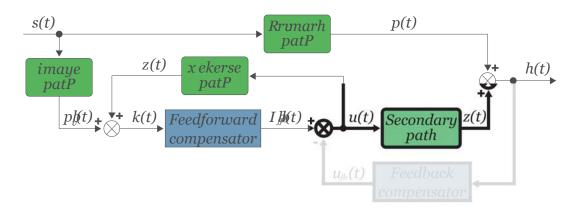
FIGURE 1.7. Reduced block diagram representation for a feedforward control problem.
