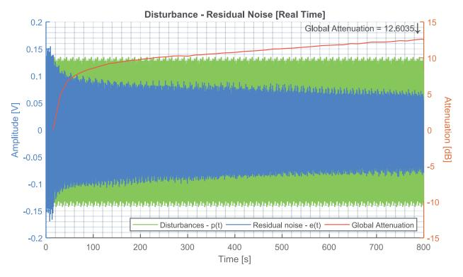
Figure 12: Performance of FUSBA FIR adaptive compensator (60 parameters, experimental).
