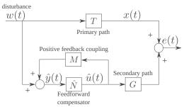
Fig. 1. Adaptive active noise feedforward compensation.
