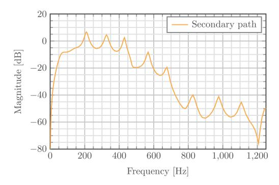
FIGURE 3.9. Identified secondary path for second test bench configuration.
