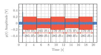
Fig. 10. Step changes in frequencies using the adaptive controller.
