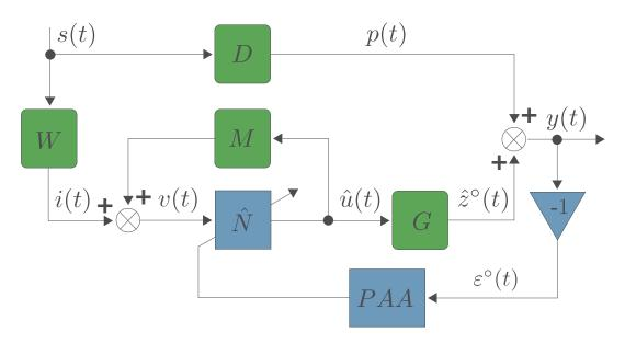
FIGURE 5.9. Feedforward control scheme with PAA.
