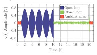
Fig. 13: Interference attenuation: residual noise in open loop and closed loop.
