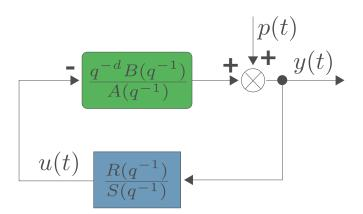
FIGURE 4.1. Feedback regulation scheme.
