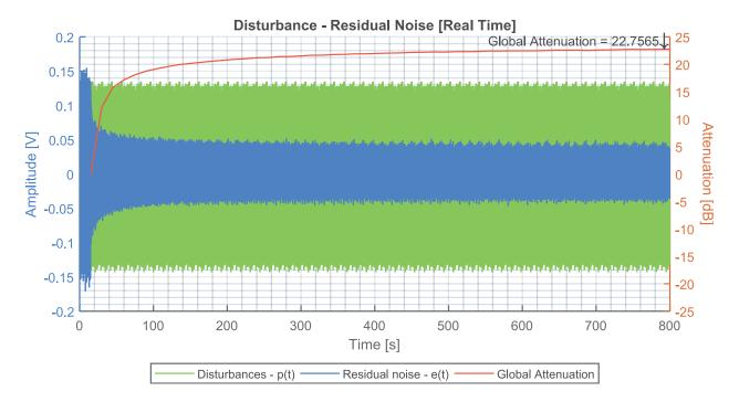
Figure 10: Performance of YK FIR adaptive compensator with 60 parameters (experimental).
