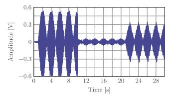
Acoustic interference attenuation using a robust controller. Noise frequencies: 170 + 170.5 Hz and 285 + 285.5 Hz then 180 + 180.5 Hz and 295 + 295.5 Hz. Loop closed at 10 s.
