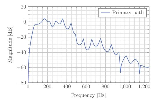
FIGURE 3.5. Identified primary path for first test bench configuration.
