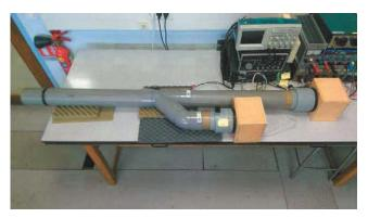
Fig. 1. Duct ANC test bench (photograph).
