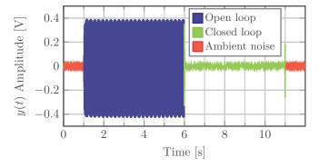
Fig. 11: Real-time experiment results: tonal disturbances.
