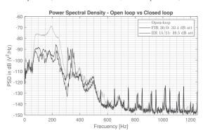
Fig. 8. PSD comparison of FIR 30/0 and IIR 15/15 standard adaptive compensators using FUSBA matrix adaptation (70-270 Hz disturbance, 600 s experiments).
