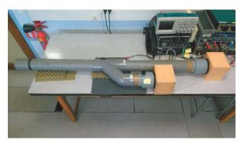
Fig. 2. Active noise control test bench (Photo).
