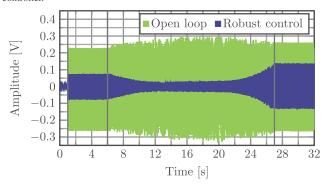
Fig. 11. Residual noise in open loop (green) and closed loop (blue) using a robust controller under the effect of tonal disturbances with variable frequencies.
