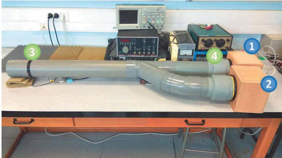
Figure 2: Duct active noise control test bench (Photo).
