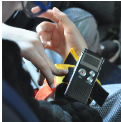
Figure 14.2: The second version of the probe is worn on the wrist. It consists of a strap covered with velcro on which an audio recorder/player. It has three main buttons that are tactily recognizable, one to start recording, the second to stop recording and the third to play the last recording.
