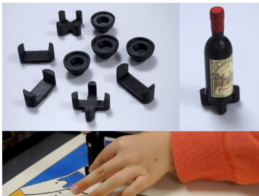
Figure A.3: The conductive supports designed for the interactive map.
