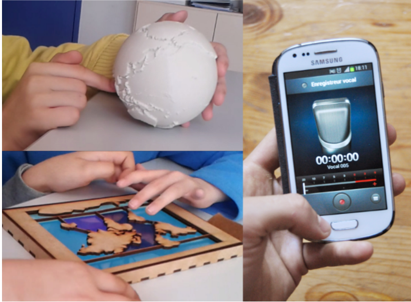
Figure A.1: Probes designed in January 2015. Top left: a 3D printed tactile globe. Bottom left: a tablet with a laser cut overlay, creating an interactive map. Right: an audio-recorder app.
