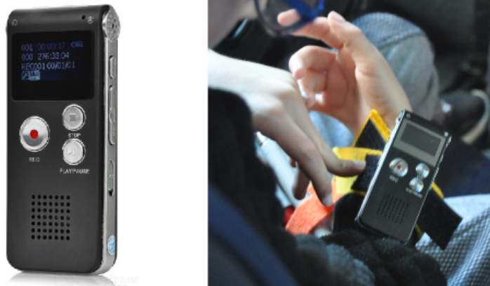
Figure 14.2: The second version of the probe is worn on the wrist. It consists of a strap covered with velcro on which an audio recorder/player. It has three main buttons that are tactily recognizable, one to start recording, the second to stop recording and the third to play the last recording.
