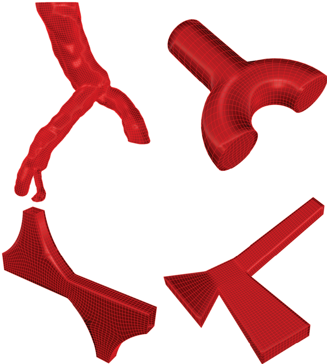
Figure 4.15: Optimized quadrilateral meshes computed from an aligned global parameterization and a geometry-feature-aware pants-to-cuboid decomposition.
